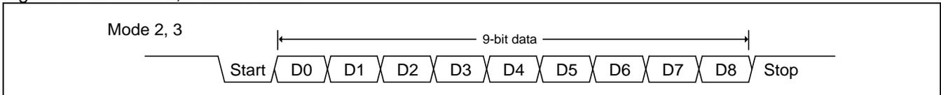
**Mode 3:** Mode 3 is the same as Mode 2 except the baud rate is variable.
