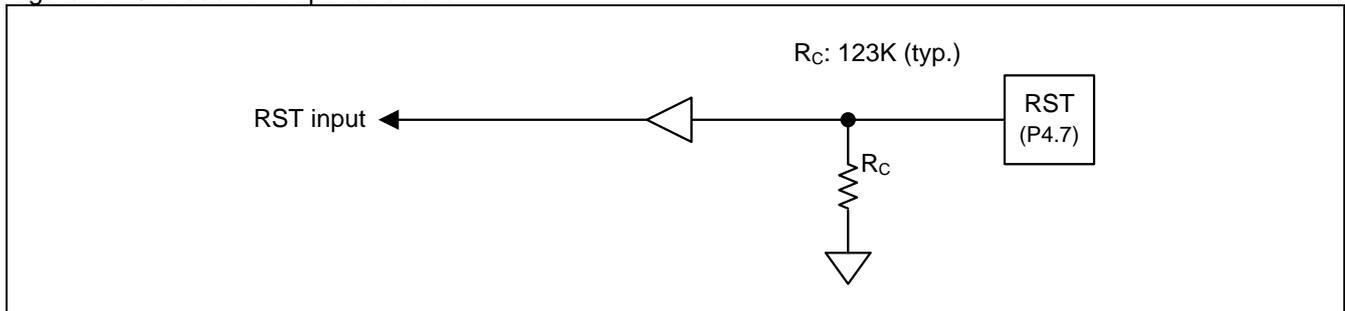
The Reset Pin also can be set as output pin, its structure is shown in [Figure 14–10](#)
