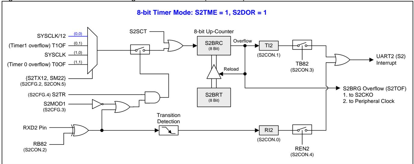
Figure 20–5. S2BRG Clock Output (S2BRG for UART Mode)
