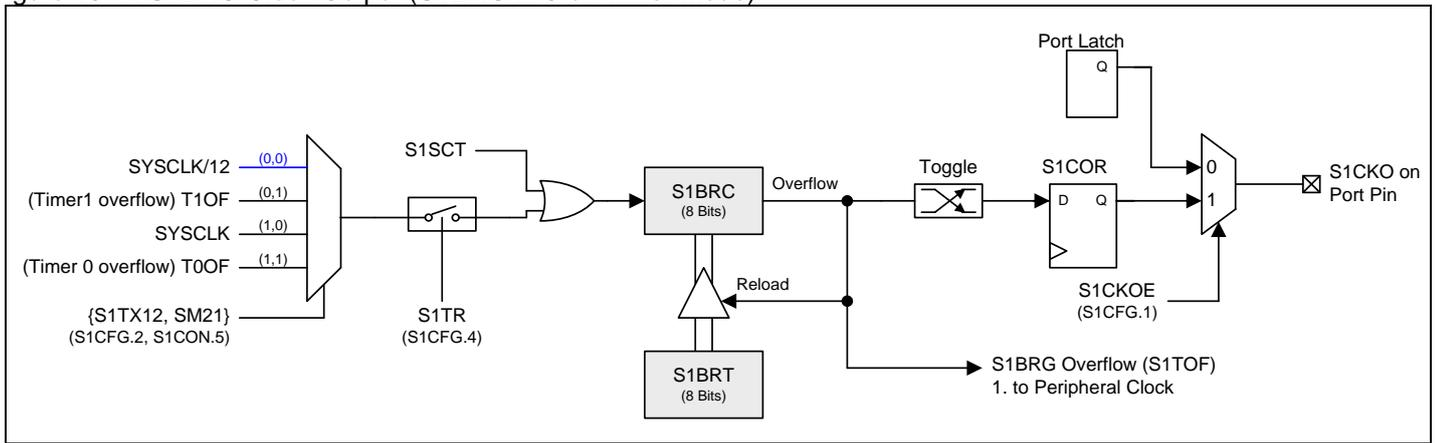
Figure 19–8. S1BRG Clock Output (S1BRG for UART Mode)
