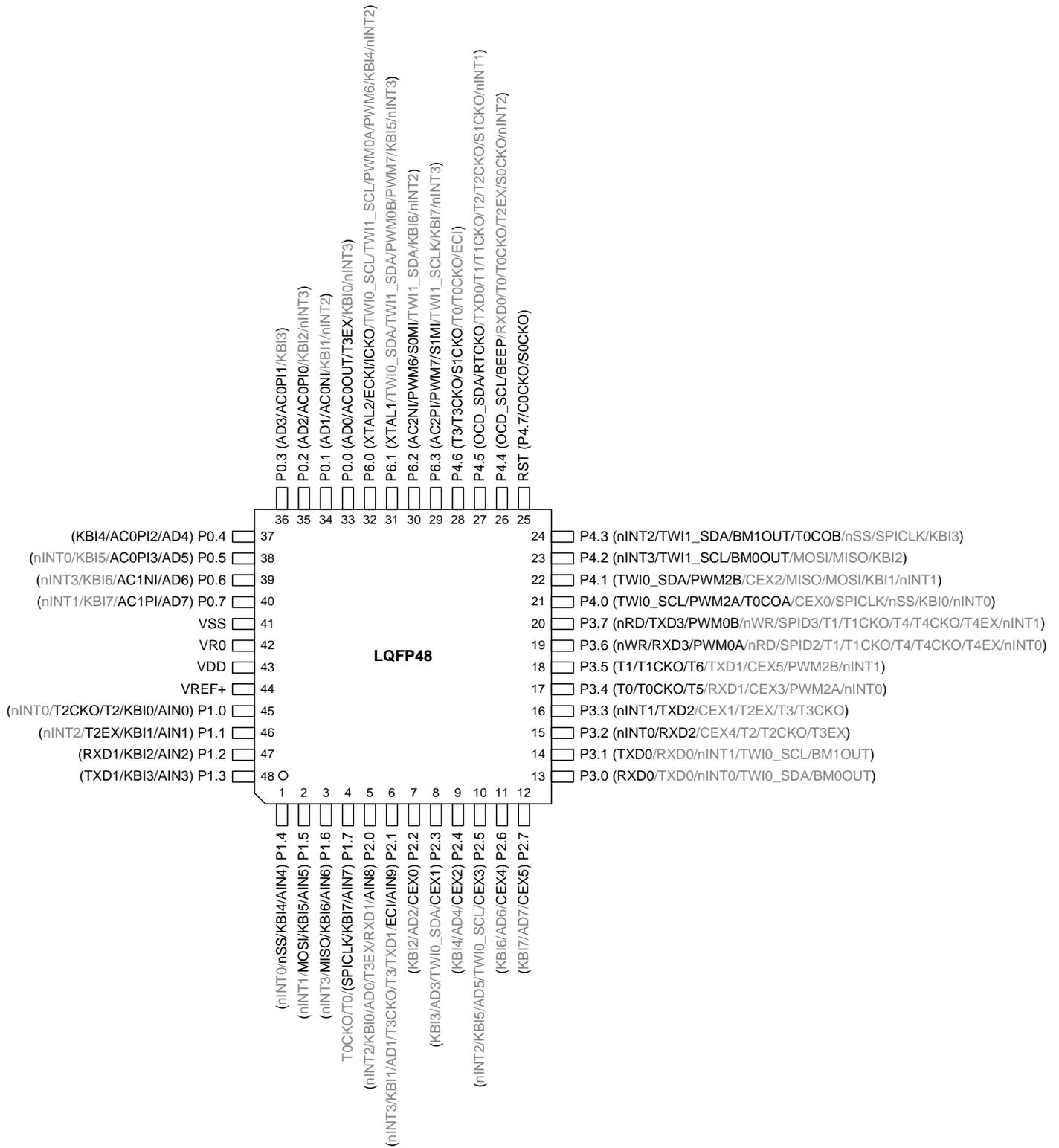
Figure 4–3. MG82F6D32AD48 LQFP48 Top View
