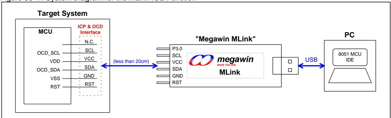
Figure 36–8. System Diagram for the ICE Function
