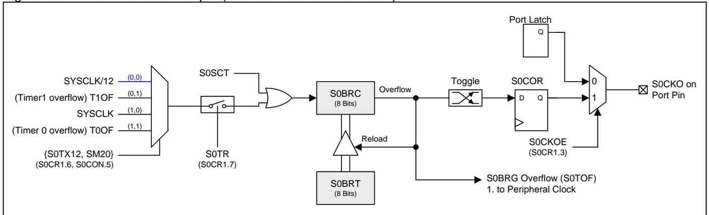
Figure 18–18. S0BRG Clock Output (S0BRG for UART Mode)
