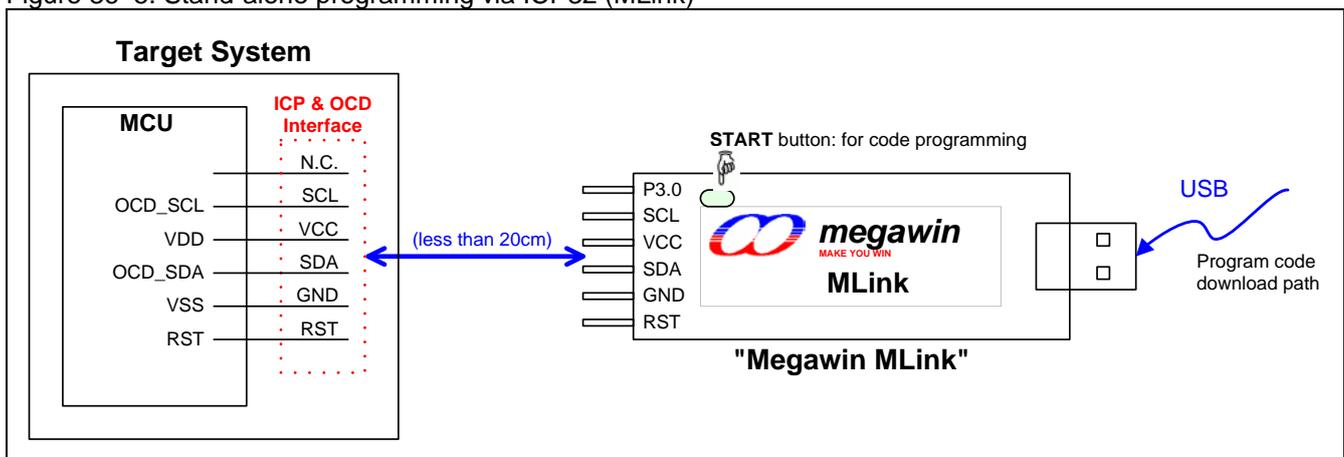
Figure 36-6. Stand-alone programming via ICP (8051 OCD ICE Adapter)
