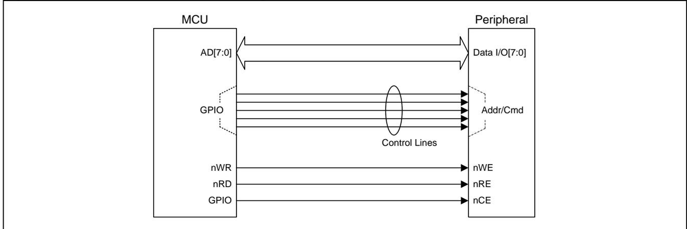
Figure 6–6. No Address Phase EMB for 8-bit Data Access
