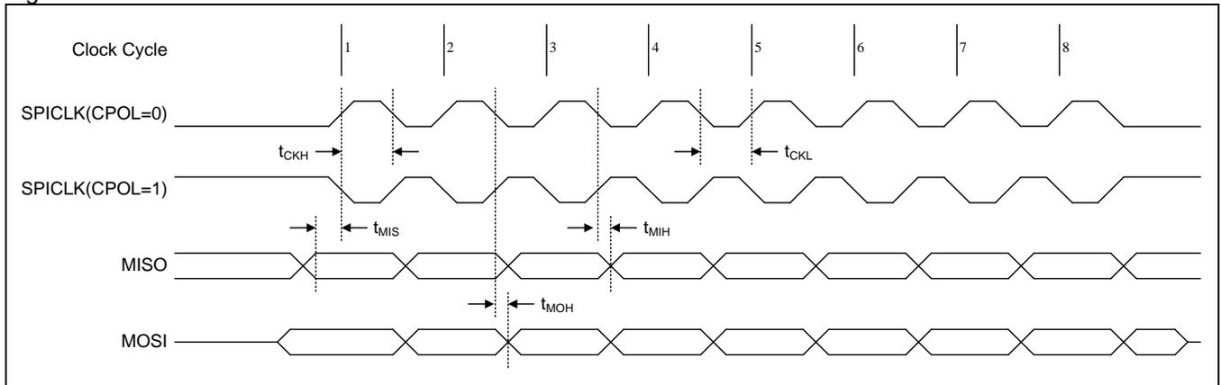
Figure 37–4. SPI Master Transfer Waveform with CPHA=1
