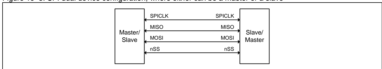
Figure 19–3. SPI dual device configuration, where either can be a master or a slave
