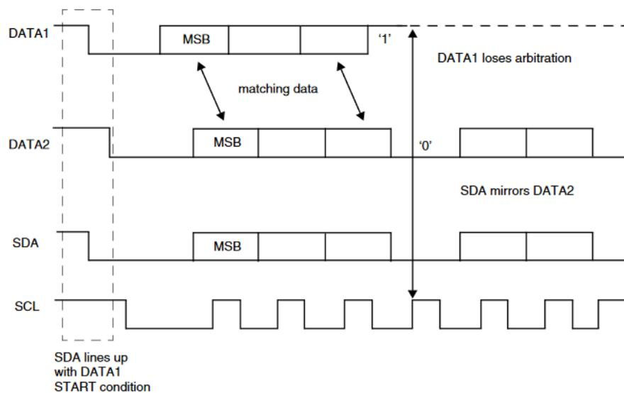
For high-speed mode, the arbitration cannot go into the data phase because each master is programmed with a unique high-speed master code. This 8-bit code is defined by the system designer and is set by writing to the High Speed Master Mode Code Address Register, IC\_HS\_MADDR. Because the codes are unique, only one master can win arbitration, which occurs by the end of the transmission of the high-speed master code.
