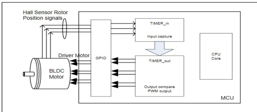
**Figure 16-30. Hall sensor timing between two timers**
