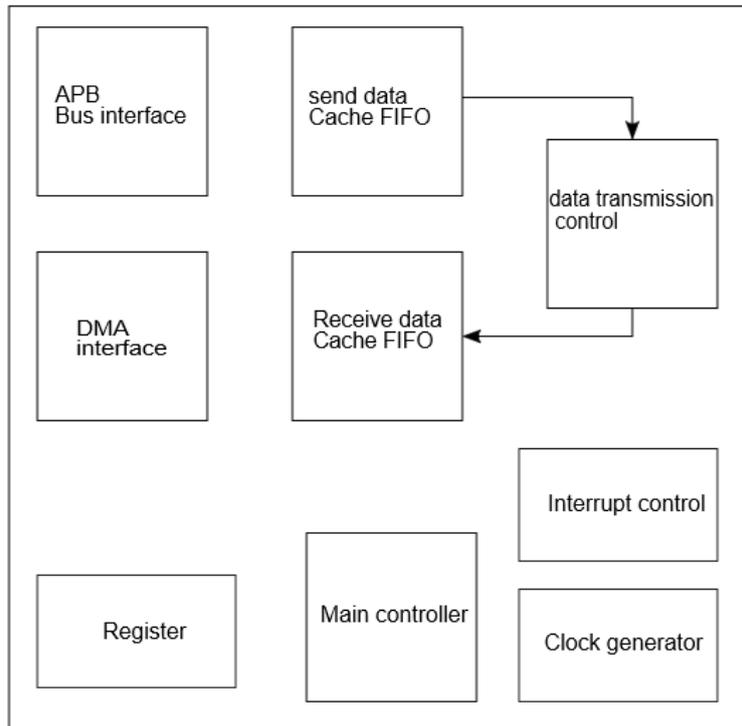
**Figure 23-2. SPI connection diagram**
