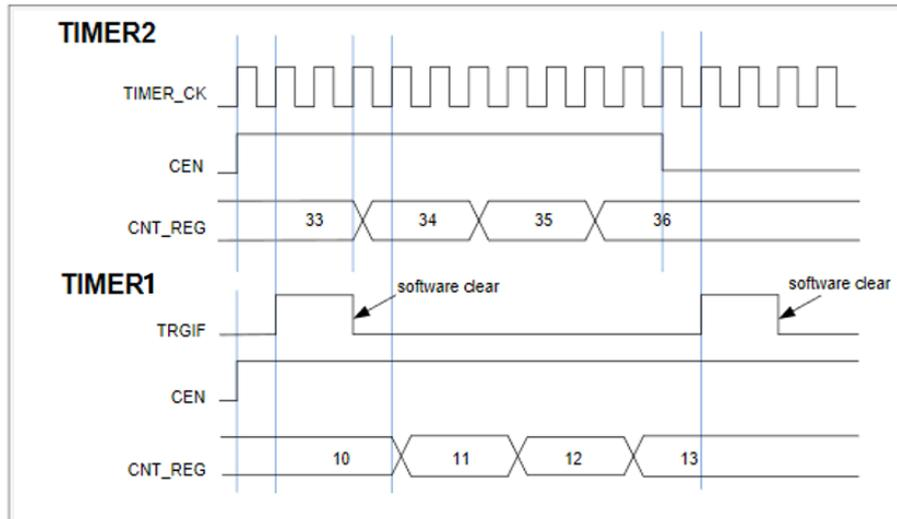
In this example, we also can use O1CPRE as trigger source instead of enable signal output. Do as follow:
