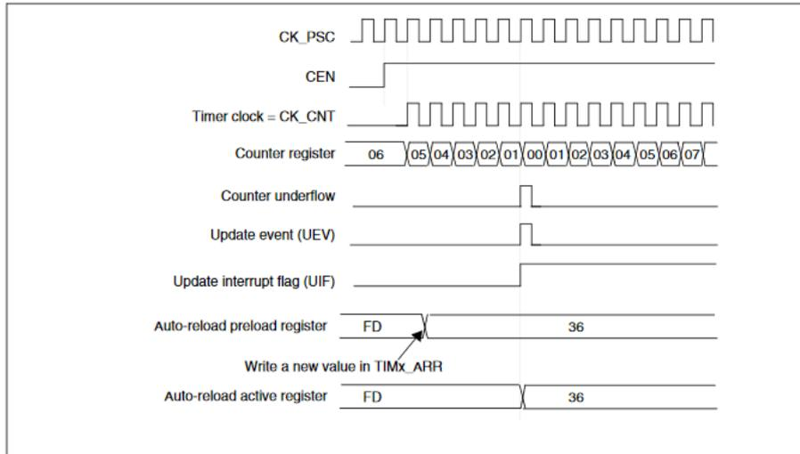
Figure 16-19. Center-aligned counter timechart, update event with ARPE=1 (counter overflow)
