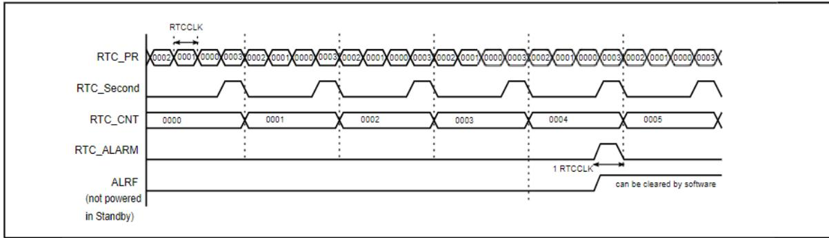
**Figure 18-3. RTC second and overflow waveform example (RTC\_PSC= 3)**
