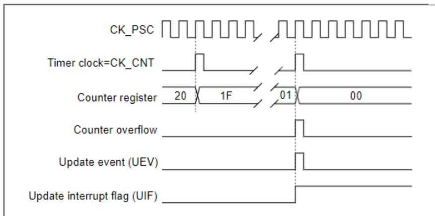
**Figure 17-18. Center-aligned counter timechart, update event with ARPE=1 (counter underflow)**
