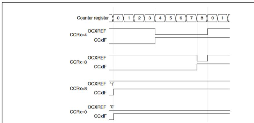
The CAPWM period is determined by 2\*TIMx\_ARR, and duty cycle is by 2\*TIMx\_CCRx. The figure below shows the CAPWM output and interrupts waveform.
