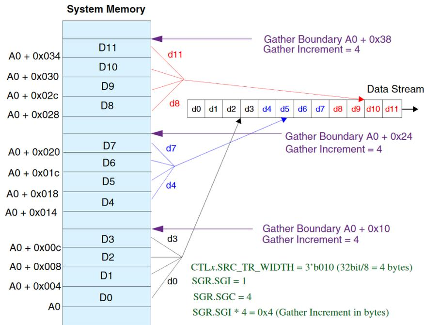
In general, if the starting address is A0 and CTLx.SINC = 2'b00 (increment source address control), then the transfer will be:
