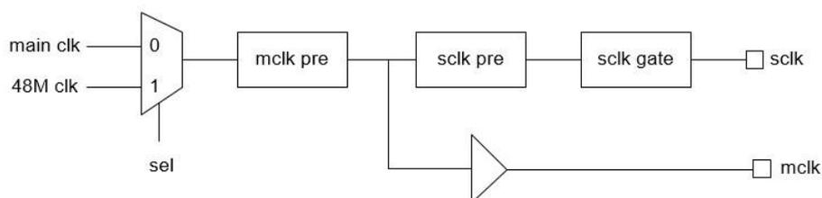
The MCLK clock source can choose from Main CLK or 48MHz clock, configured through the MCLKSRC of the RCC modules. The MCLK prescaler can be configured via the MCLKPRE of the RCC module. The prescaler of SCLK can be configured via the I2SPRE of the RCC module. Please refer to the relevant section of the RCC module for details.
