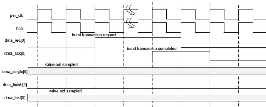
When the peripheral request DMA, the signal “dma\_req” will be asserted (assert “dma\_single\_req” for DMA single transfer). If the channel assigned to this peripheral can be granted by the arbiter, the data transfer starts, and DMAC asserts the signal “dma\_ack”. When all the data transfers are finished, the devices will stop requesting by de-assert “dma\_req”. Then DMAC will de-assert the “dma\_ack” in the next cycle. The DMA transfer
