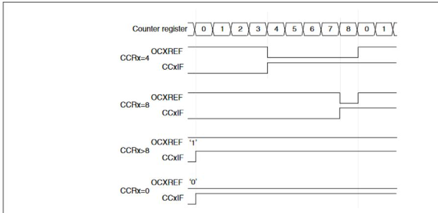
The CAPWM period is determined by  $2 \cdot \text{TIMx\_ARR}$ , and duty cycle is by  $2 \cdot \text{TIMx\_CCR}_x$ . The figure below shows the CAPWM output and interrupts waveform.
