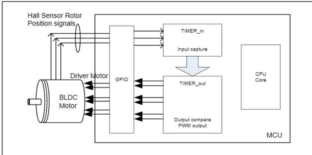
**Figure 17-27. Hall sensor timing between two timers**
