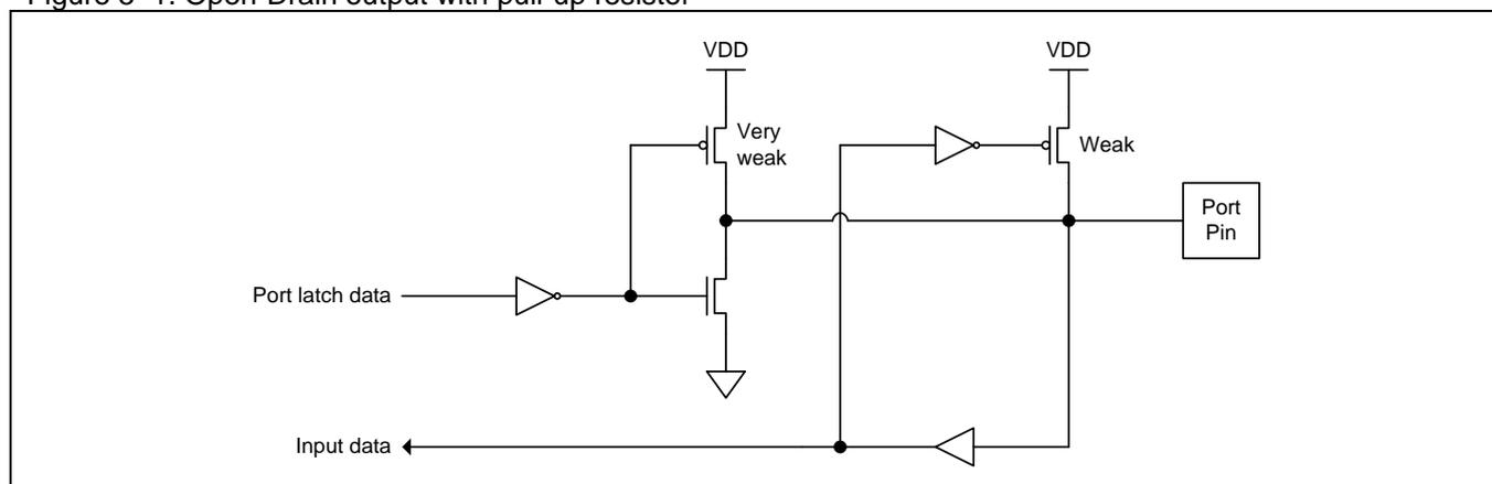
Especially for the quasi-bidirectional port pin, its configuration is illustrated in [Figure 5–2](#). The output high will have one clock driving by push-pull mode output to enhance rising time, then keep the port pin state by pull-up resistors, weak & very weak. This configuration exists on GPIO8/9/A.
