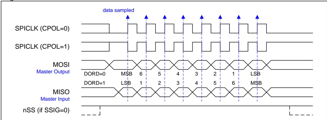
Figure 18-9. SPI Master Transfer Format with CPHA=1
