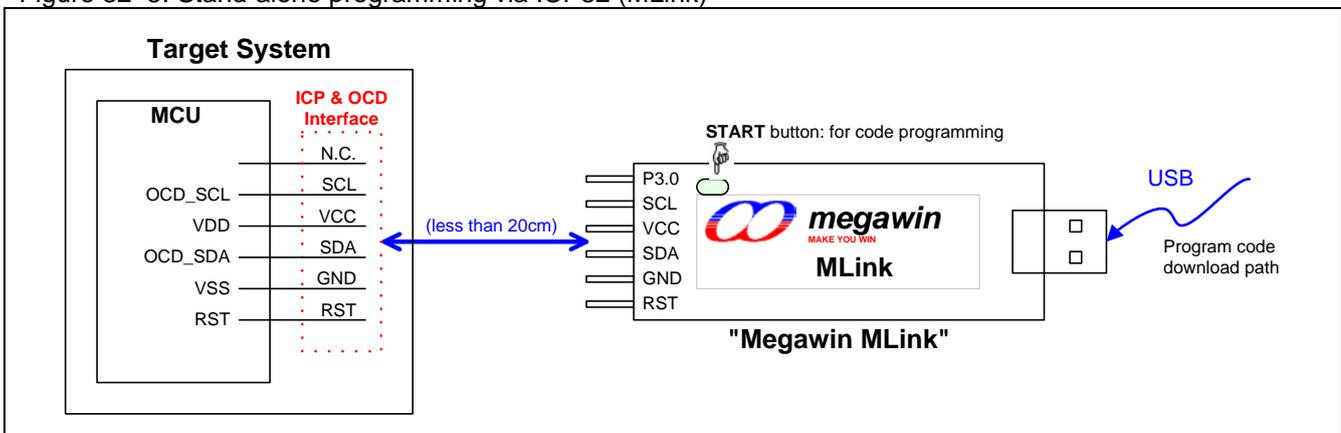
Figure 32-6. Stand-alone programming via ICP
