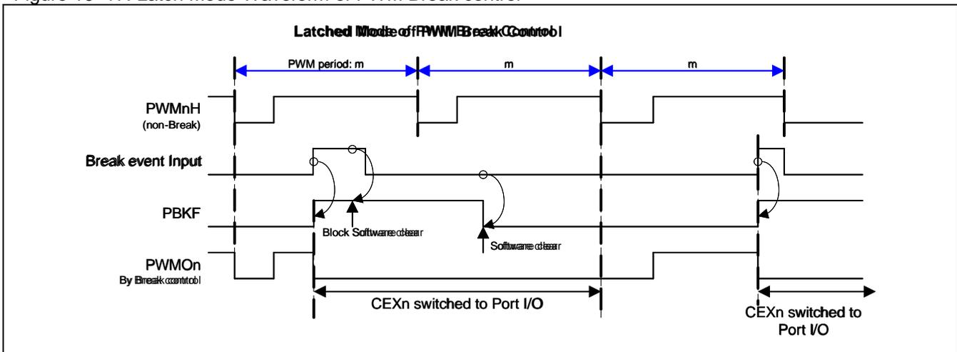
Figure 16–18. Cycle-by-Cycle Mode Waveform of PWM Break control
