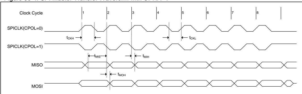
Figure 33-5. SPI Slave Transfer Waveform with CPHA=0
