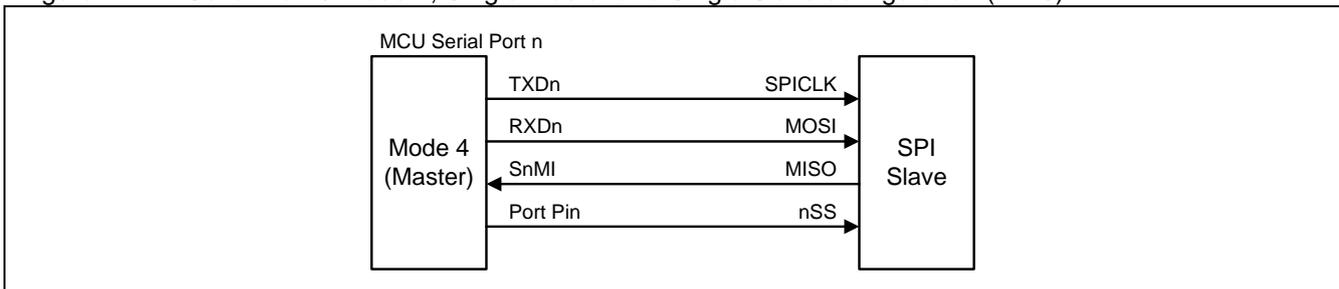
Figure 17-12. Serial Port 0 Mode 4, Single Master and Multiple Slaves configuration (n = 0)
