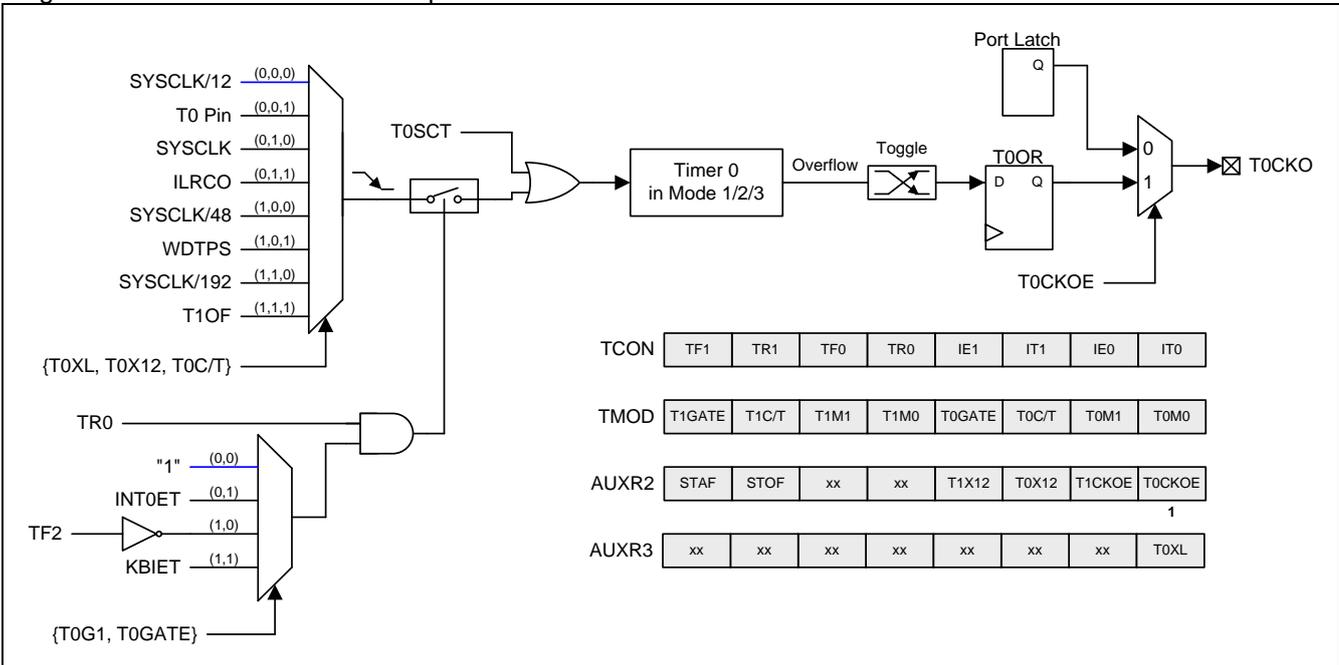
Figure 15-11. Timer 1 in Clock Output Mode
