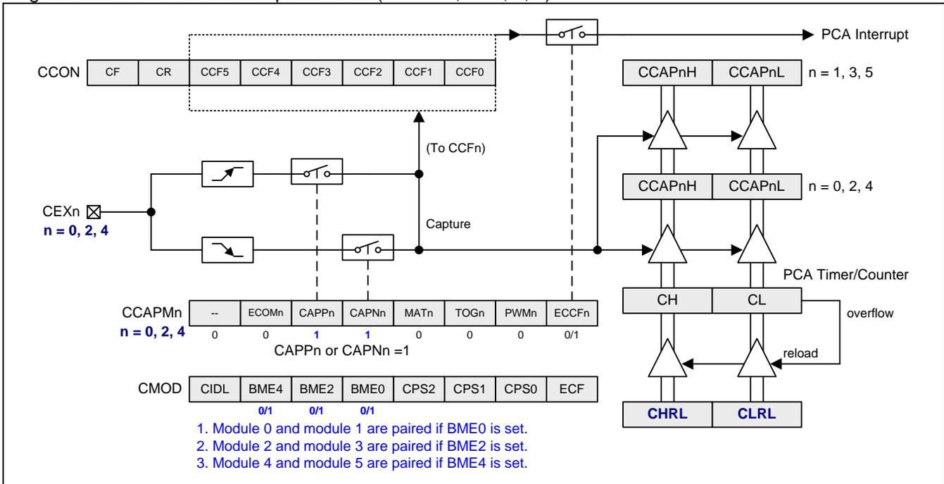
Figure 16-6. PCA0 Buffered Capture Mode Waveform
