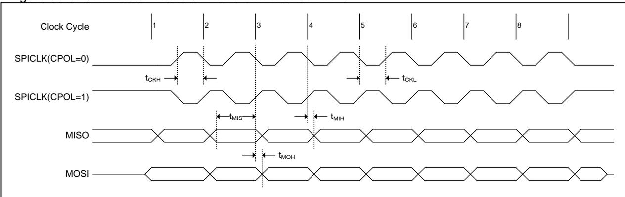
Figure 33-4. SPI Master Transfer Waveform with CPHA=1
