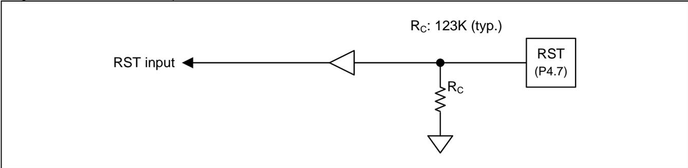
The Reset Pin also can be set as output pin, its structure is showed in Figure 13–11
