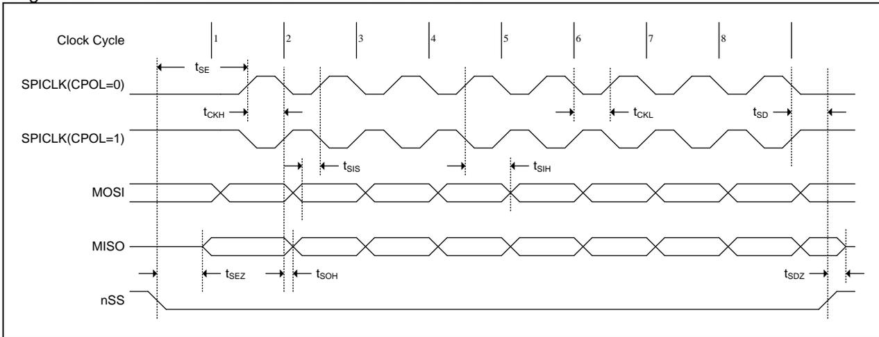
Figure 33-6. SPI Slave Transfer Waveform with CPHA=1
