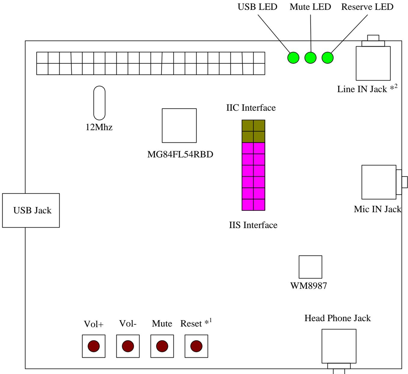
\*<sup>1</sup> Will trigger the MG84FL54RBD into ISP area for DFU ( Device Firmware Upgrade ) function
