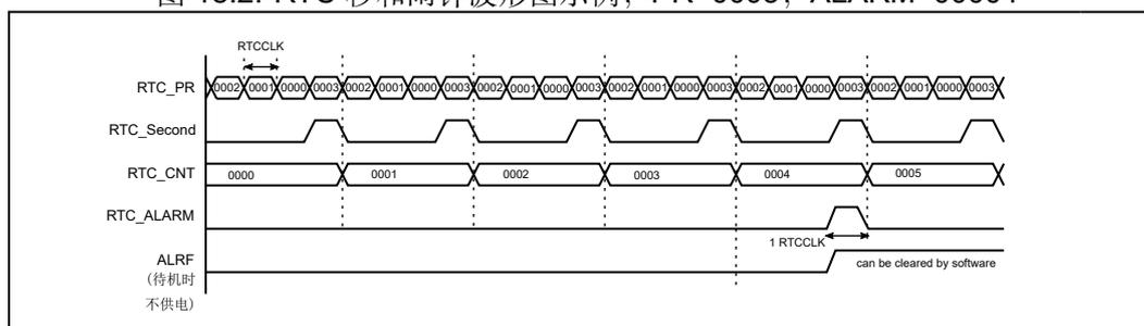
图 18.3: RTC 溢出波形图示例, PR=0003
