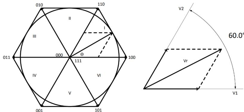
图 19.6.2 : SVPWM Representation in an Orthogonal Plane
