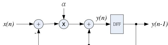
$$\alpha = \frac{\omega_c T_s}{1 + \omega_c T_s} \quad \begin{aligned} \omega_c &: \text{cutoff angular frequency of filter} \\ T_s &: \text{sampling period} \end{aligned}$$
