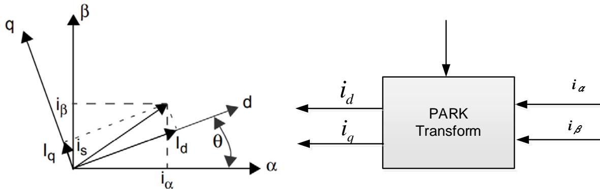
$$\begin{aligned} I_d &= I_\alpha \cdot \cos \theta_r + I_\beta \cdot \sin \theta_r \\ I_q &= -I_\alpha \cdot \sin \theta_r + I_\beta \cdot \cos \theta_r \end{aligned}$$
