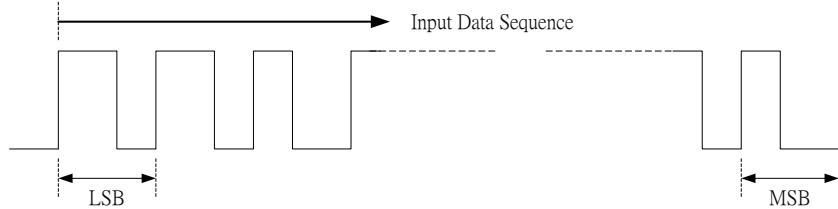
IR\_DEC\_SET[6] (DOUT\_REV) = 1 : first input data is MSB
