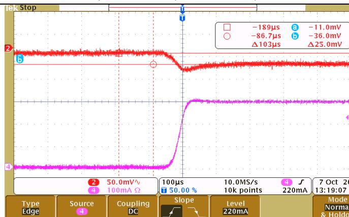
Fig 1. Load Transient (1mA to 300mA)
