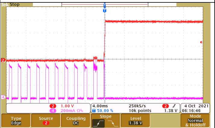
Fig 6.  $V_{OUT}$  short to GND and release
