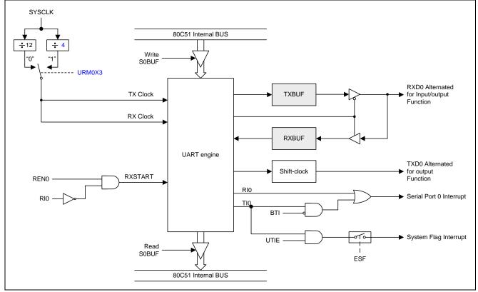
Figure 18-3. Serial Port 0 Mode 0
