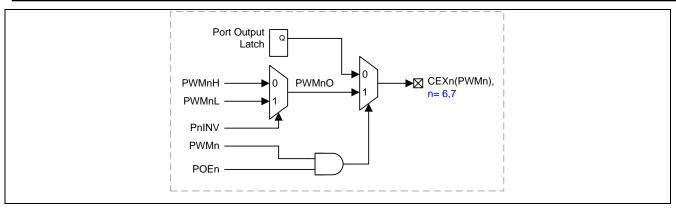
POEM0 in **MGEQ1C064** controls the POEn output timing to align with PWM cycle. The configuration and waveform of the aligned function is shown in Figure 17–21.
