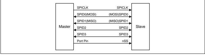
Figure 22–10. QPI single master & single slave configuration
