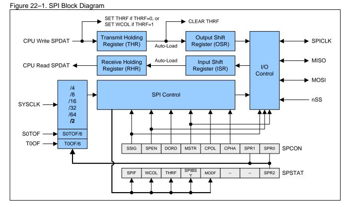
The SPI interface has four pins: MISO, MOSI, SPICLK and nSS:
