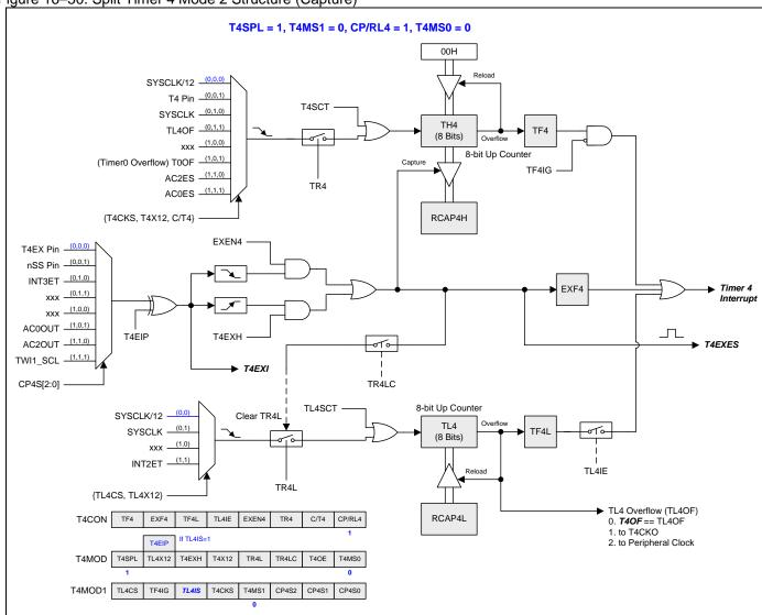
Figure 16-50. Split Timer 4 Mode 2 Structure (Capture)
