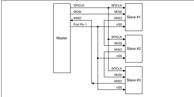
Figure 22–9. SPI slave in Daisy-Chain configuration
