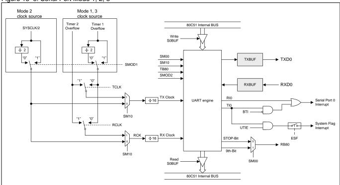
Figure 18-6. Serial Port Mode 1, 2, 3
