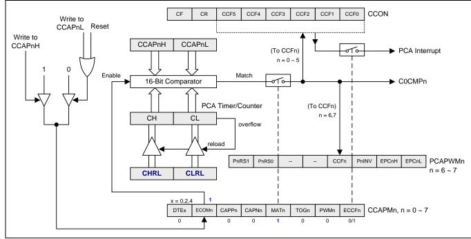
Figure 17–7. PCA Software Timer Mode
