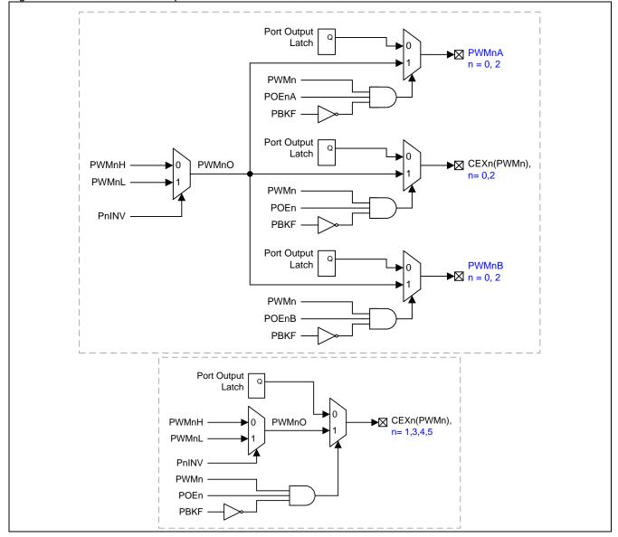
Figure 17–20. PCA Module output control
