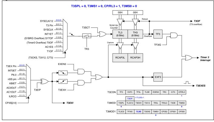
Figure 16-31. Timer 3 Mode 2 Structure (Capture Mode)
