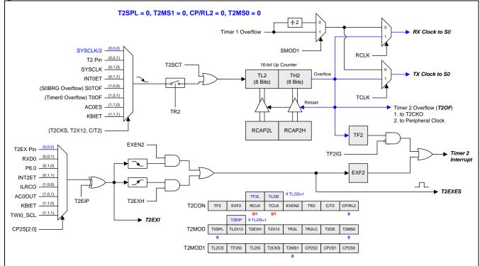
Figure 16–23. Timer 2 in Baud-Rate Generator Mode
