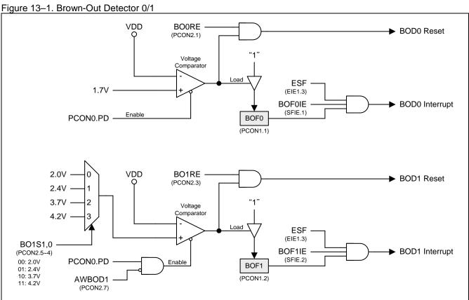
To reduce power consumption, software may clear EBOD1 (PCON2.2) to disable BOD1 if the BOD1 is not applied in user application.
