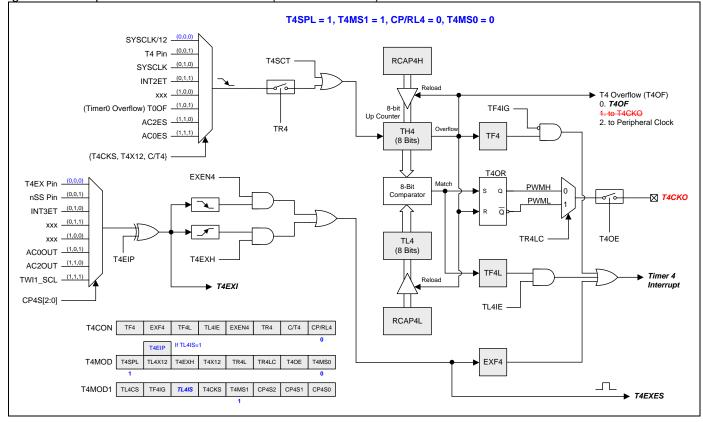
Figure 16–52. Split Timer 4 Mode 4 Structure (8-bit PWM mode)
