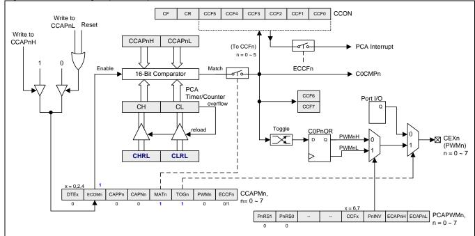
Figure 17-8. PCA High Speed Output Mode
