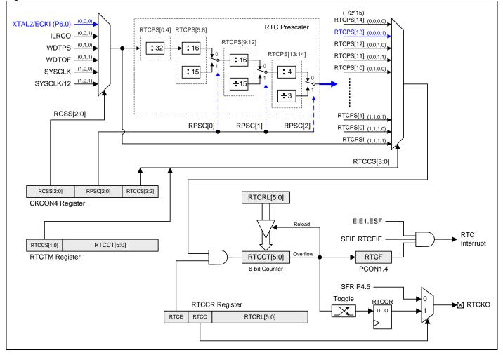
Figure 11–1. Real-Time-Clock Counter
