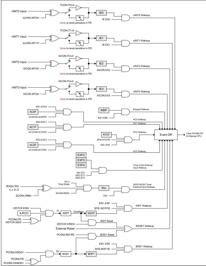
Figure 13–2. Wakeup structure of Power Down mode
