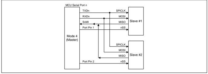
The SPI master satisfies the transfer with the full function SPI module of Megawin MG82/84 series MCU with CPOL, CPHA and DORD selection. For CPOL and CPHA condition, **MGEQ1C064** uses an easy way by initialize SPI clock assigned port pin (TXD0) polarity to fit them. Table 18–41 shows the serial port Mode 4 mapping with the four SPI operating mode.
