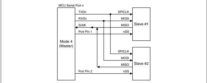
The SPI master satisfies the transfer with the full function SPI module of Megawin MG82/84 series MCU with CPOL, CPHA and DORD selection. For CPOL and CPHA condition, **MGEQ1C064** uses an easy way by initialize SPI clock polarity to fit them. Table 18–13 shows the serial port Mode 4 mapping with the four SPI operating mode.
