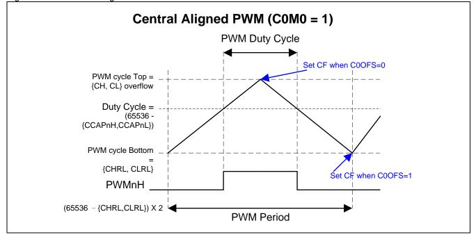
Figure 17–22. Central Aligned PWM with Variable Resolution
