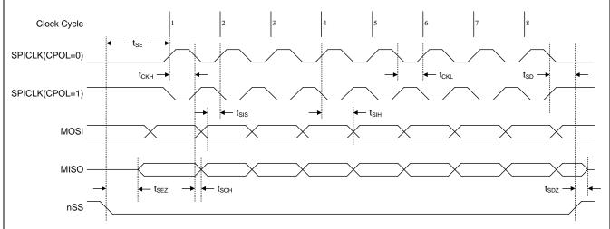
Figure 37-6. SPI Slave Transfer Waveform with CPHA=1
