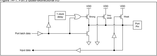
Figure 14–1. Port 3 Quasi-Bidirectional I/O
