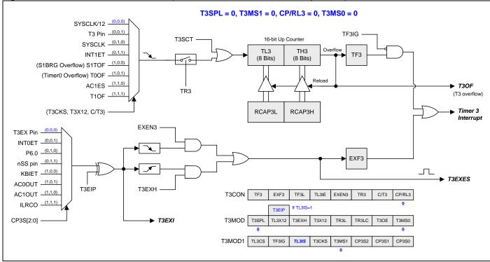
Figure 16–29. Timer 3 Mode 0 Structure (Auto-Reload and Exteranl Interrupt Mode)
