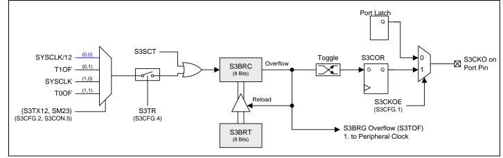
Figure 21–5. S3BRG Clock Output (S3BRG for UART Mode)
