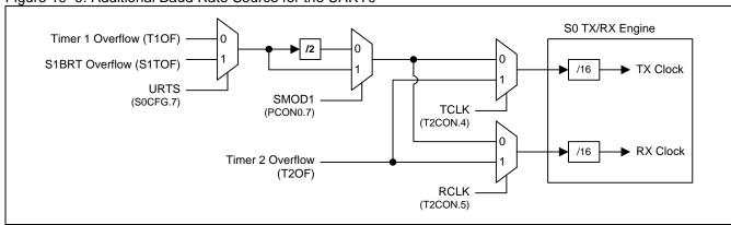
Figure 19–9. Additional Baud Rate Source for the UART0
