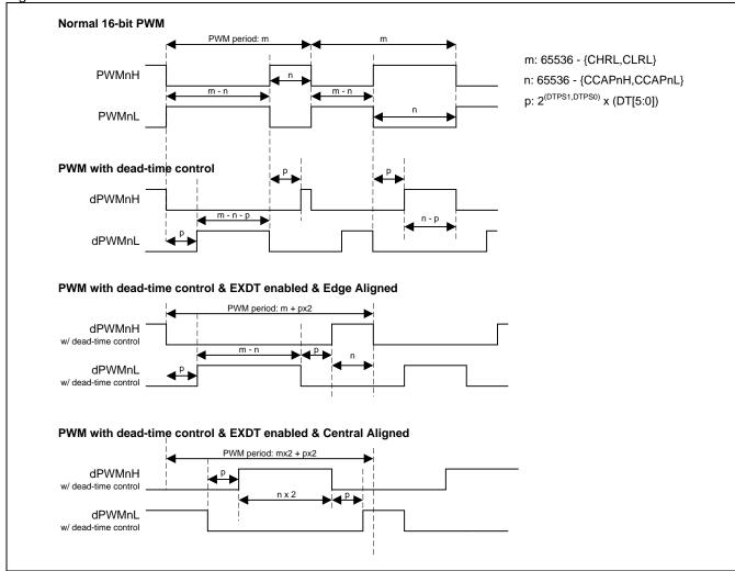
Figure 17–15. PWM Waveform with Dead-Time Control
