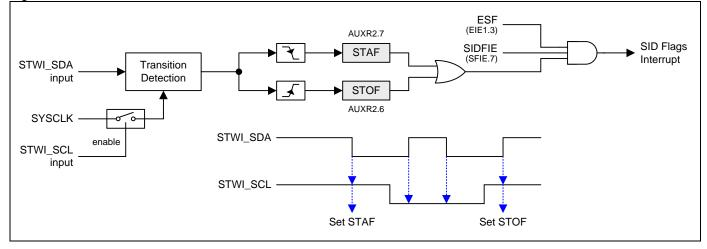
Figure 24-1. Serial Interface Detection structure
