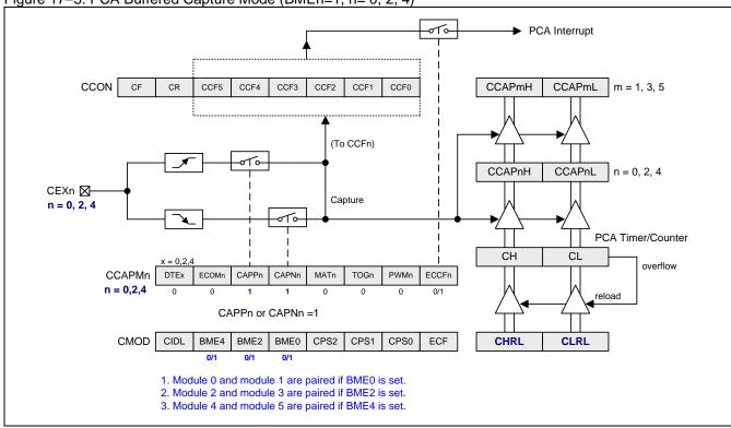
Figure 17–5. PCA Buffered Capture Mode (BMEn=1, n= 0, 2, 4)
