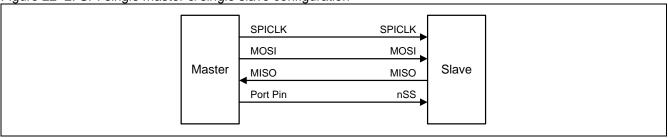
Figure 22–2. SPI single master & single slave configuration
