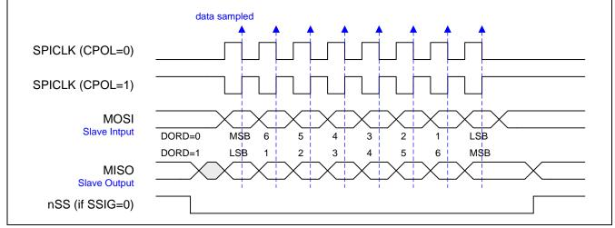
Figure 22–7. SPI Master Transfer Format with CPHA=0 data sampled SPICLK (CPOL=0) SPICLK (CPOL=1) MOSI Master Output DORD=0 MSB 6 5 4 3 2 1 LSB DORD=1 LSB 6 MSB 1 2 3 4 5 MISO Master Input i. nSS (if SSIG=0) \_ \_ \_ J  $\square$   $\_$   $\_$   $\_$  .
