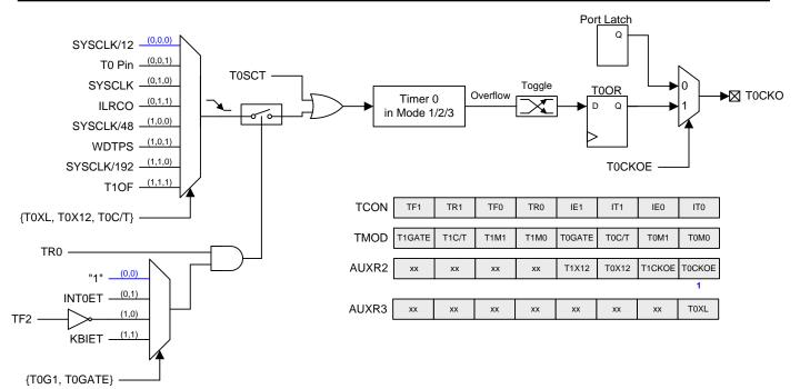
Figure 16–11. Timer 0 Clock Output Control
