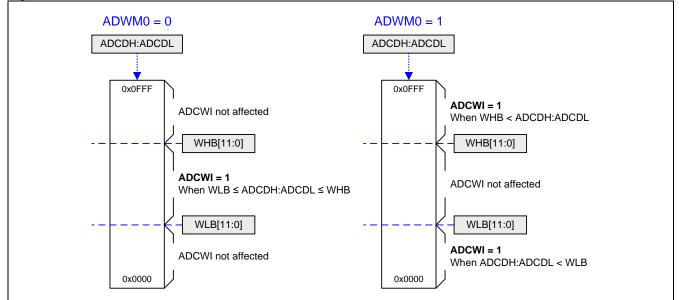
Figure 29-4. ADC Window Detect
