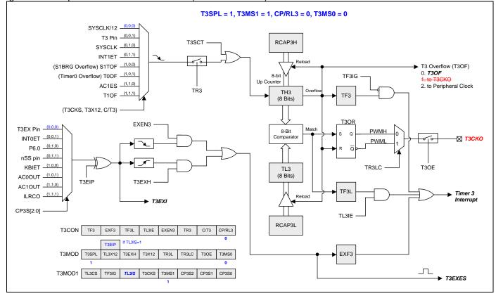
Figure 16–38. Split Timer 3 Mode 4 Structure (8-bit PWM mode)
