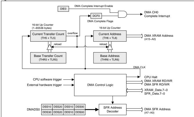
Figure 8–2. DMA Structure
