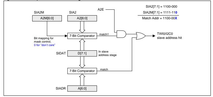
Figure 23-3. Multiple slave address recognition
