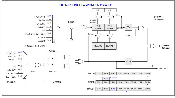
Figure 16-45. Timer 4 Mode 2 Structure (Capture Mode)
