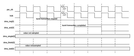
When the peripheral request DMA, the signal "dma\_req" will be asserted (assert "dma\_single\_req" for DMA single transfer). If the channel assigned to this peripheral can be granted by the arbiter, the data transfer starts, and DMAC asserts the signal "dma\_ack". When all the data transfers are finished, the devices will stop requesting by de-assert "dma\_req". Then DMAC will de-assert the "dma\_ack" in the next cycle. The DMA transfer
