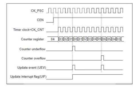
Figure 16-14. Center-aligned counter timechart, PSC=0
