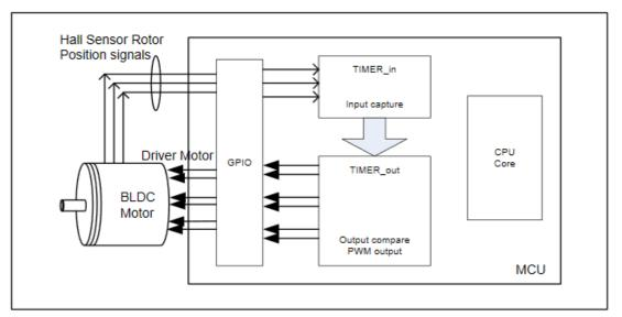
Figure 17-26. Hall sensor is used to BLDC motor
