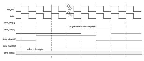
Figure 14-3. DMA single data transfer
