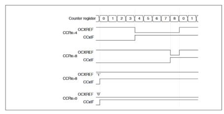
Figure 16-23. EAPWM waveforms (ARR=8)
