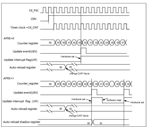
Figure 17-8. Up-counter timechart, change TIMx\_ARR on the go
