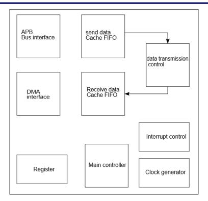
Figure 23-2. SPI connection diagram
