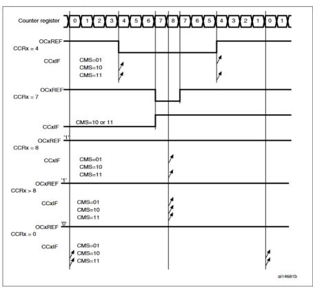
Figure 17-23. CAPWM waveforms (ARR=8)
