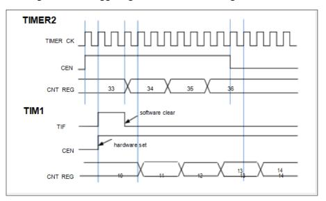
In this example, we also can use update Event as trigger source instead of enable signal.
