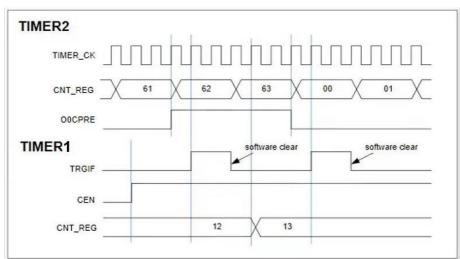
Figure 16-36. Pause Timer1 with O1CPREF signal of Timer2
