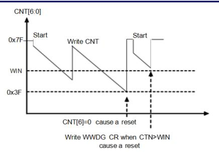
Calculate the WWDG timeout by using the formula below.
