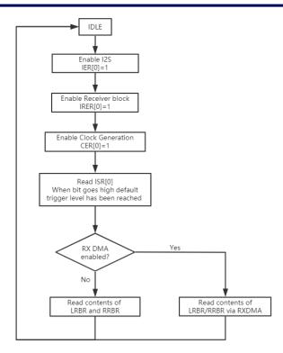
The reason why the clock generator is finally turned on is that the transmission of the series starts from the WS change, and the I2S needs to be configured before this.
