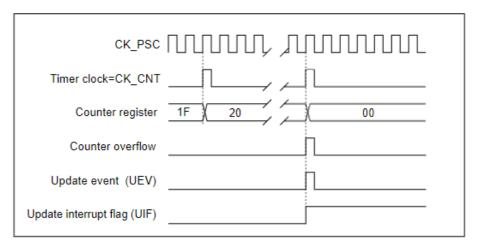
Figure 16-8. Up-counter timechart, change TIMx\_ARR on the go
