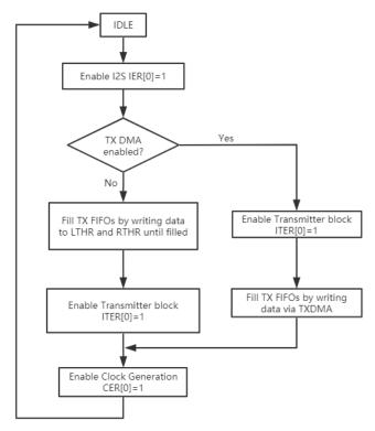
The reason why the clock generator is finally turned on is that the transmission of the series starts from the WS change, and the I2S needs to be configured before this.
