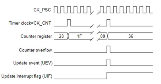
Figure 16-13. Down-counter timechart, change TIMx\_ARR on the go (APRE=0)
