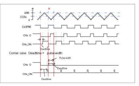
Figure 16-25. Complementary output with dead-time insertion
