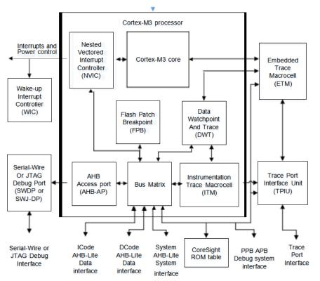
Figure 2-1. The structure of the Cortex<sup>™</sup> -M3 processor
