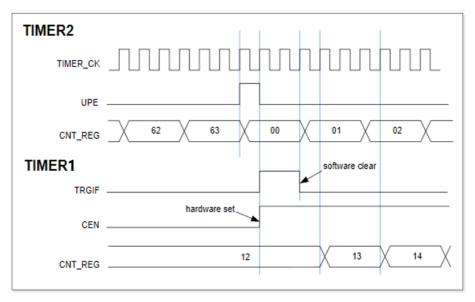
■ Enable Timer1 count with Timer2's enable/O1CPRE signal
