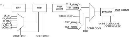
Figure 16-21. Input capture logic
