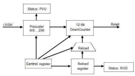
The free watchdog is enabled by writing the value 0xCCCC in the control register (IWDG\_KR), and the counter starts counting down. When the counter reaches the value 0x000, a reset is generated.
