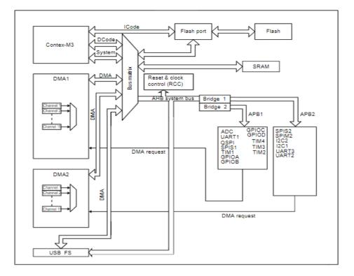
Figure 2-2. MG32F10xx Medium-density series system architecture
