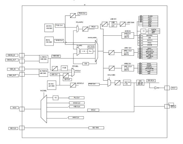
The system clock "MAINCLK" acts as the clock source of AHB, APB, USB and I2S. The clock source of Cortex SysTick and TRACE is AHB clock divided by 8.
