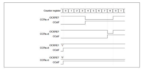
Figure 17-22. EAPWM waveforms (ARR=8)
