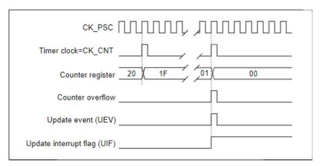
Figure 16-18. Center-aligned counter timechart, update event with ARPE=1 (counter underflow)
