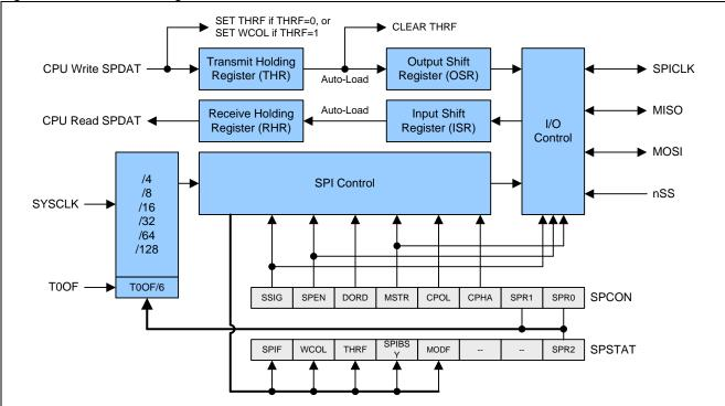
The SPI interface has four pins: MISO, MOSI, SPICLK and nSS:
