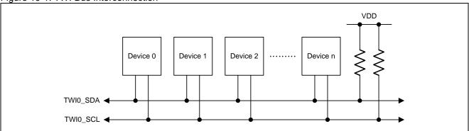
The TWI bus may operate as a master and/or slave, and may function on a bus with multiple masters. The CPU interfaces to the TWI through the following four special function registers: SICON configures the TWI bus; SISTA reports the status code of the TWI bus; and SIDAT is the data register, used for both transmitting and receiving TWI data. SIADR is the slave address register. And, the TWI hardware interfaces to the serial bus via two lines: SDA (serial data line) and SCL (serial clock line).
