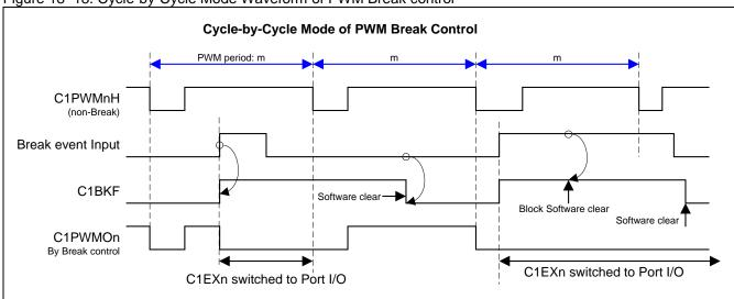
Bit 4~3: C1BKE1.1~0, PWM Break Enable 1 selection. This function is only active on CEXn output mode (n=0~5).
