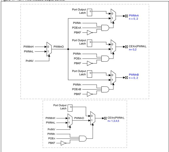
POEM0 in **MG82F6P32** controls the POEn output timing to align with PWM cycle. The configuration and waveform of the aligned function is shown in Figure 17–19.
