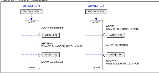
Another application of ADC Window Detect is to specify the voltage is lager or less than a specific voltage. For example:
