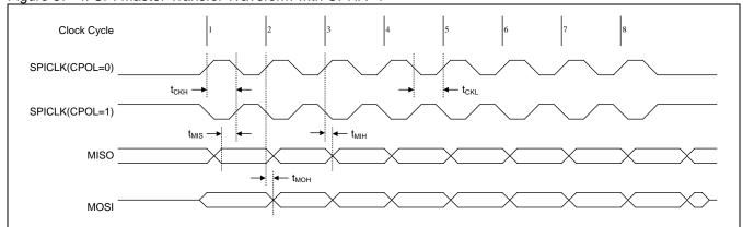
Figure 37–5. SPI Slave Transfer Waveform with CPHA=0
