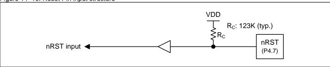
The Reset Pin also can be set as output pin, its structure is showed in Figure 14-11
