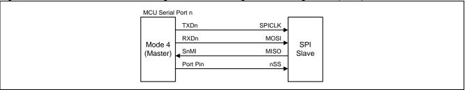
Figure 19–11. Serial Port 0 Mode 4, Single Master and Multiple Slaves configuration (n = 0)
