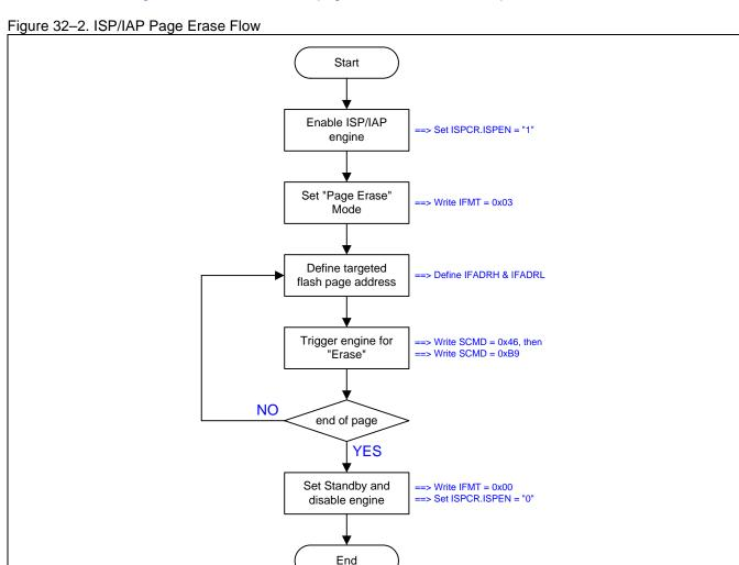
Figure 32–3 shows the demo code of the ISP/IAP page erase operation.
