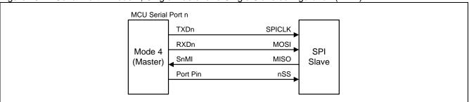
Figure 20-3. Serial Port 1 Mode 4, Single Master and Multiple Slaves configuration (n = 1)
