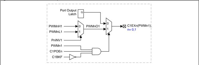
C1POEM0 in MG82F6P32 controls the C1POEn output timing to align with PWM cycle. The configuration and waveform of the aligned function is shown in Figure 17–19.
