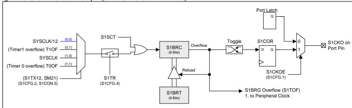
Figure 20-10. S1BRG Clock Output (S1BRG for UART Mode)
