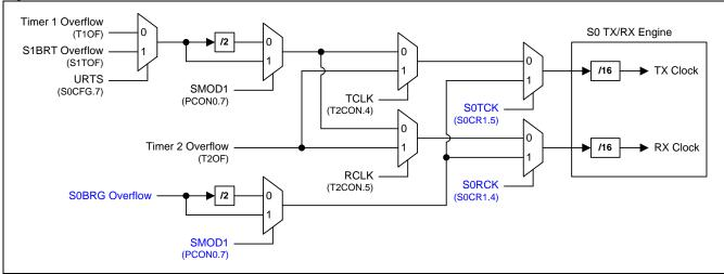
When S1BRG is used as the baud rate generator of S0, the baud rate is as follows.
