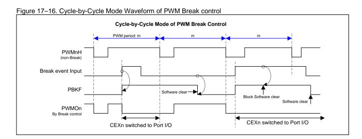
Bit 4~3: PBKE1.1~0, PWM Break Enable 1 selection. This function is only active on CEXn output mode (n=0~5).
