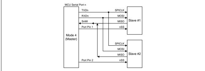
The SPI master satisfies the transfer with the full function SPI module of Megawin MG82/84 series MCU with CPOL, CPHA and DORD selection. For CPOL and CPHA condition, **MG82F6P32** uses an easy way by initialize SPI clock assigned port pin (TXD0) polarity to fit them. Table 19–2 shows the serial port Mode 4 mapping with the four SPI operating mode.
