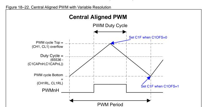
C1PWMCR: PCA1 PWM Control Register
