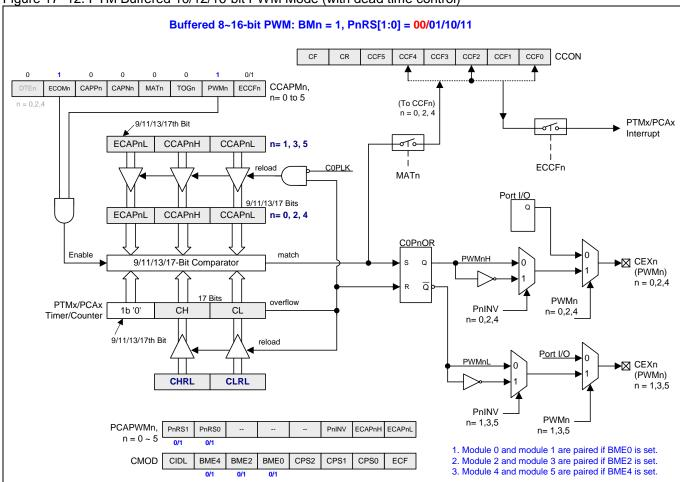
Figure 17-12. PTM Buffered 10/12/16-bit PWM Mode (with dead time control)
