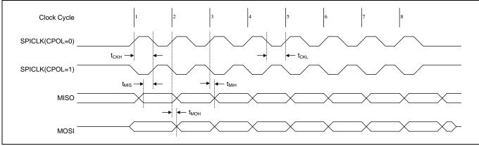
Figure 37-4. SPI Master Transfer Waveform with CPHA=1
