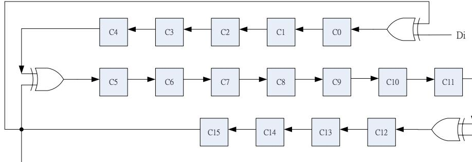
Figure 21.1 : The general LSFR architecture of CRC16-CCITT
