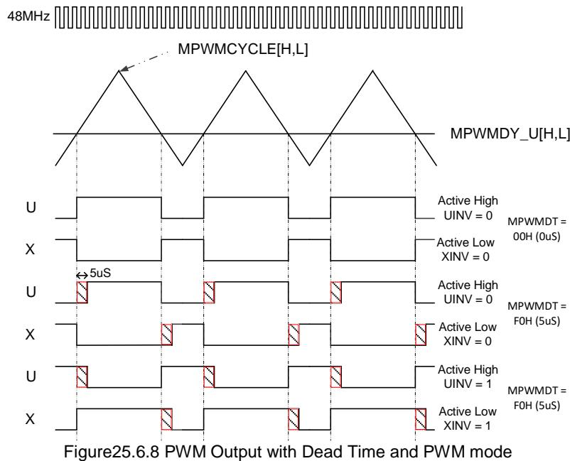
Figure25.6.8 PWM Output with Dead Time and PWM mode
