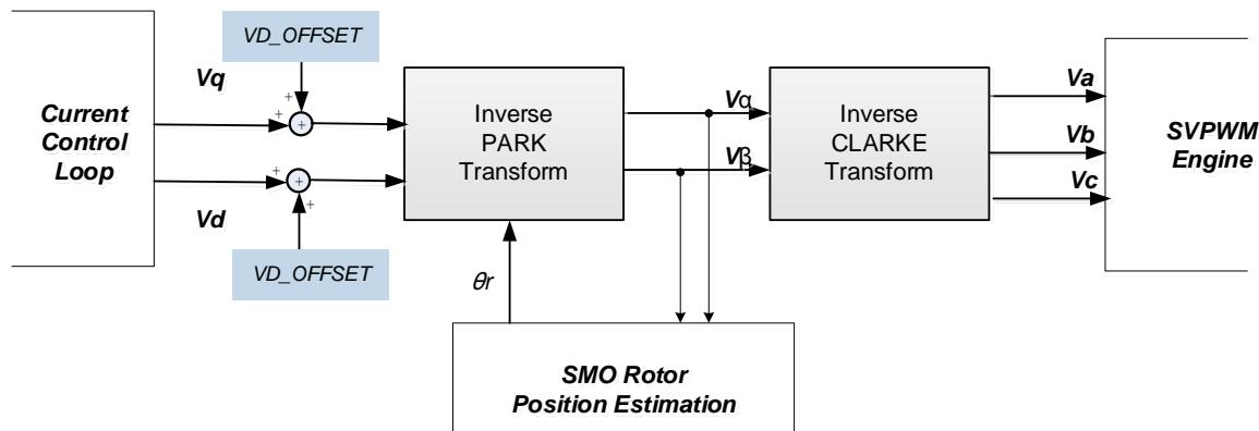
Figure 17.4.1 : Inverse Coordinate Transformation Block Architecture
