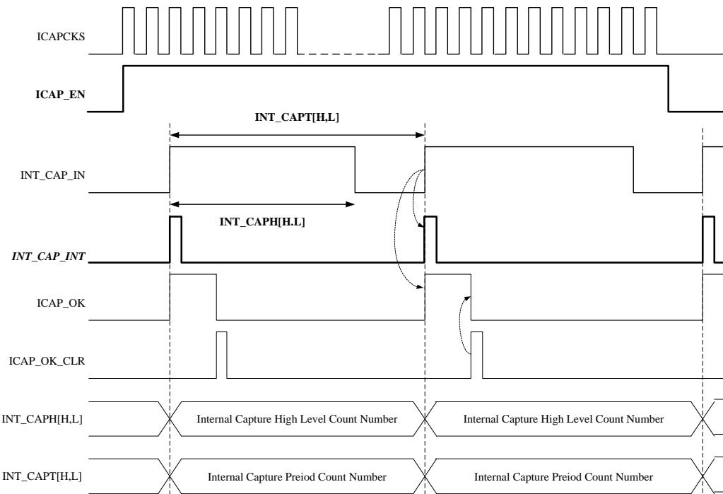
Figure 19.2.1 : The Waveform Sequence of Internal Capture
