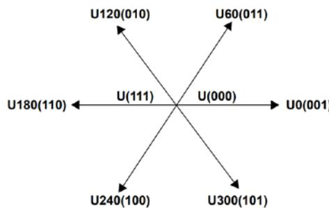
Figure 25.6.2 : Space Vector Pulse Width Modulation (SVPWM)
