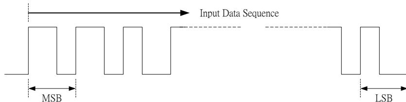
Figure 23.1.3 : The output data reverse select
