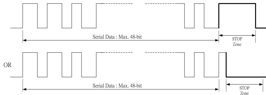
Figure 23.1.1 : The header and stop signal express
