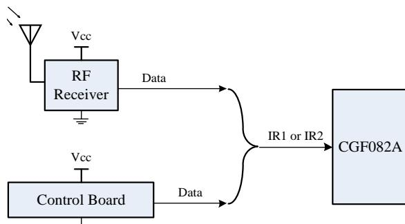
Figure 23.1 : One wire signal decode by CGF022A
