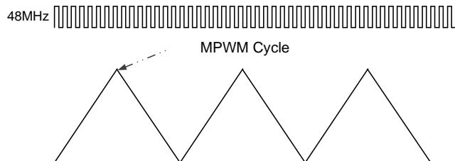
Figure25.6.6 : Motor PWM is count up and down timer
