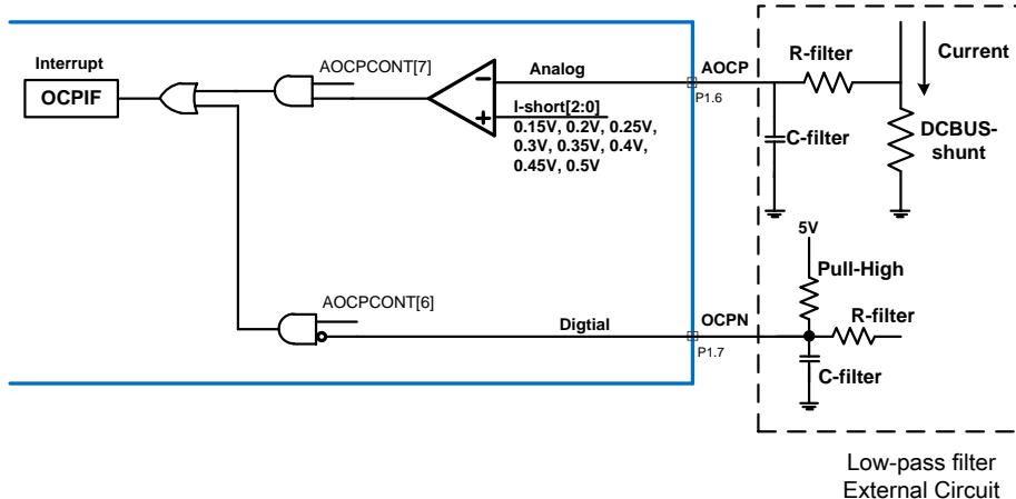
Figure 25.10.1 : Analog OCP and Digital OCPN Unit Architecture
