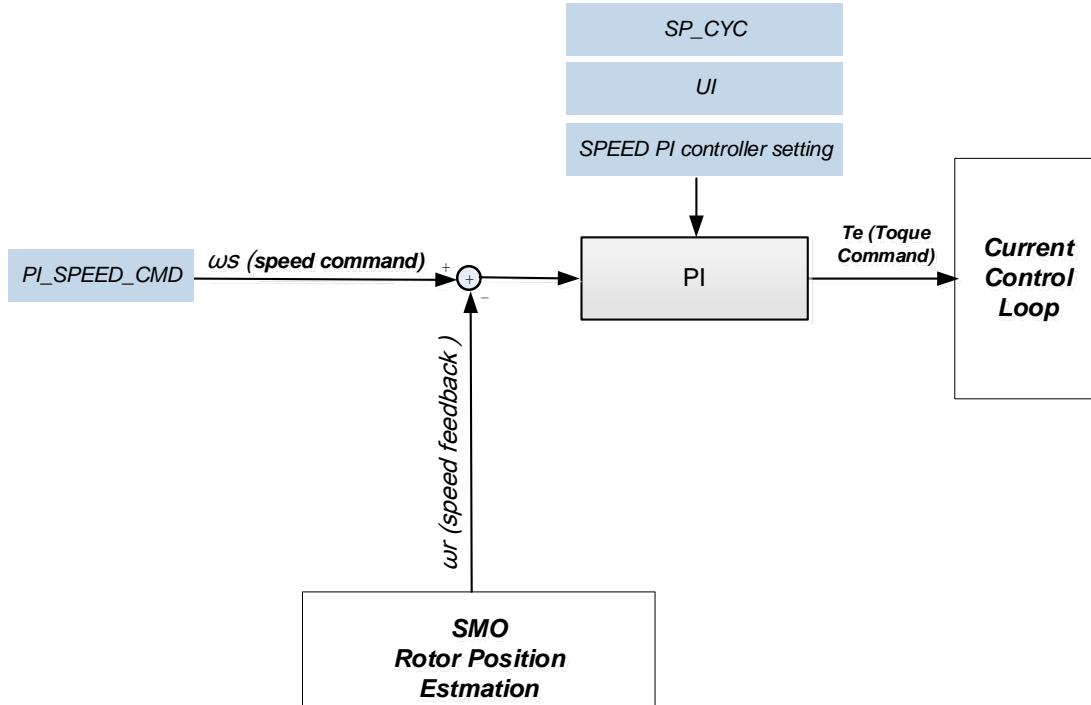
Figure 25.7.1 : Speed Control Loop Block Architecture
