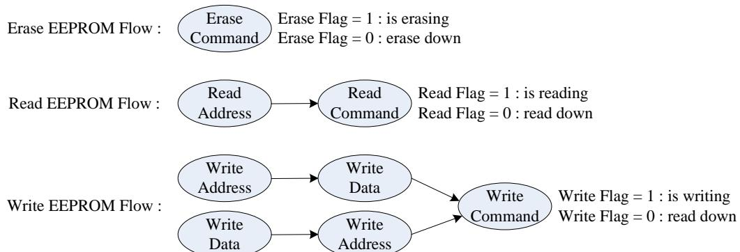
Figure 17.1 : EEPROM Erase, Read, and Write Control Flow
