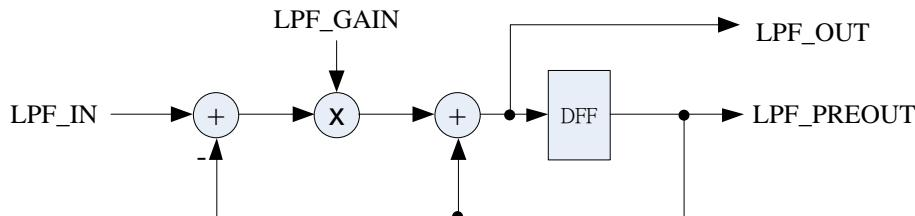
Figure 25.11.2 : LPF architecture and corresponding parameters
