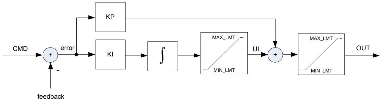
Figure 25.8.2 : User PI Block Architecture
