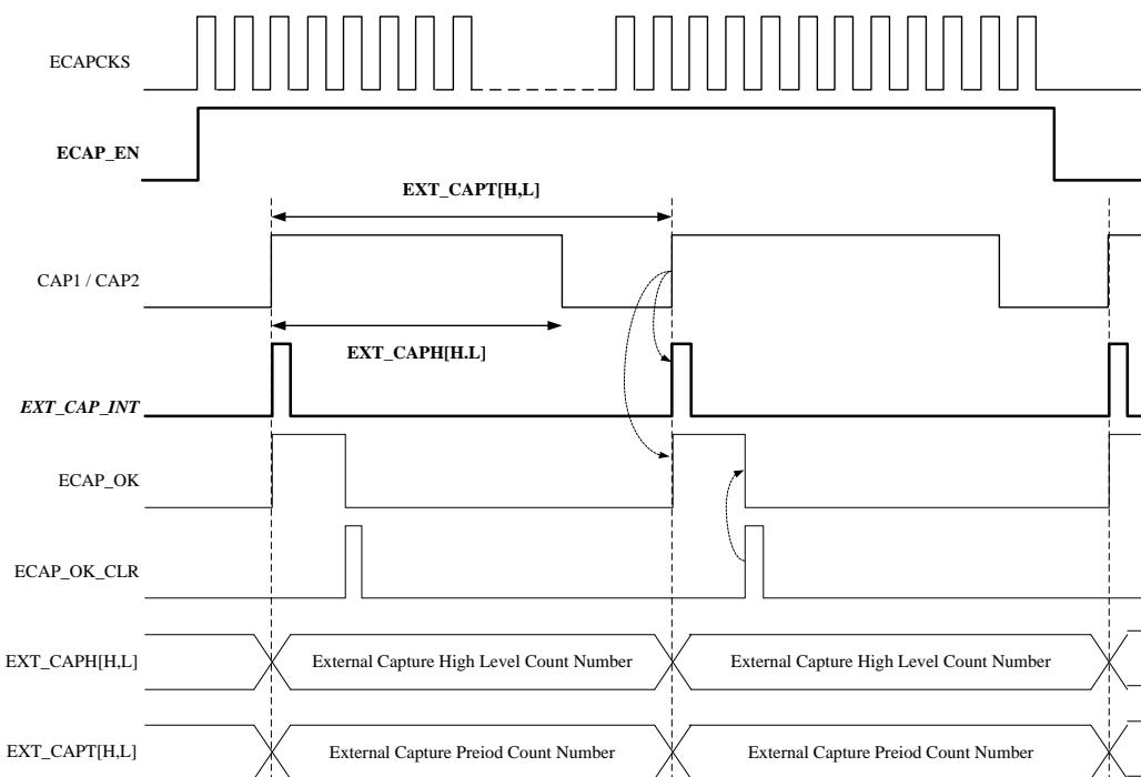
Figure 19.1.1 : The Waveform Sequence of External Capture
