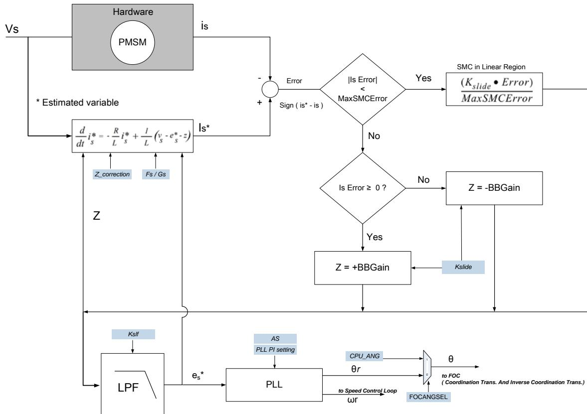
Figure 25.5.1 : SMO Rotor Position Estimation Block Architecture
