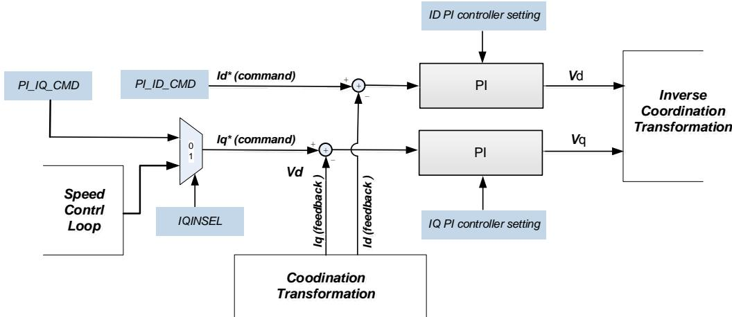
Figure 25.3.1 : Current Control Loop Block Architecture
