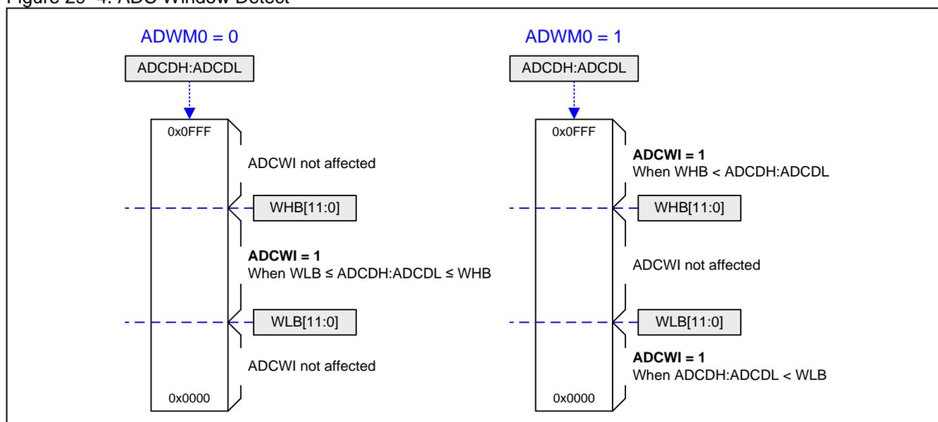
Another application of ADC Window Detect is to specify the voltage is larger or less than a specific voltage. For example:
