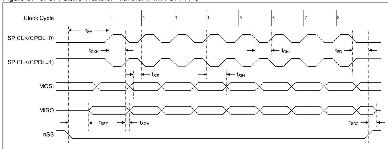
Figure 37–6. SPI Slave Transfer Waveform with CPHA=1
