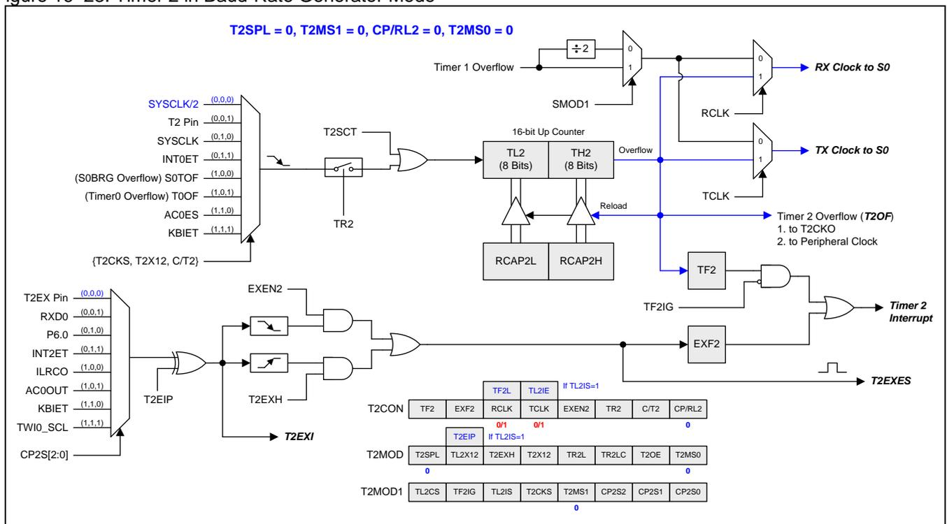
Figure 16–24. Split Timer 2 in Baud-Rate Generator Mode
