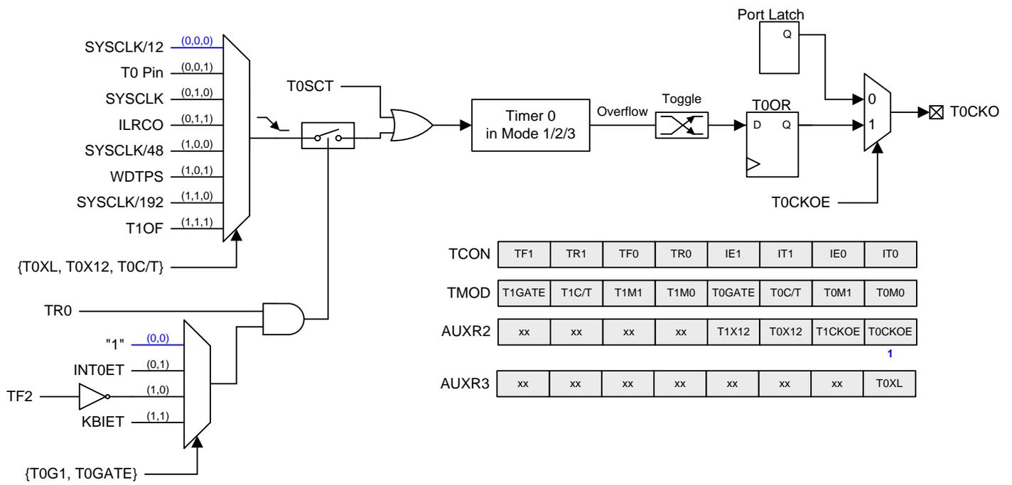
Figure 16–11. Timer 0 Clock Output Control
