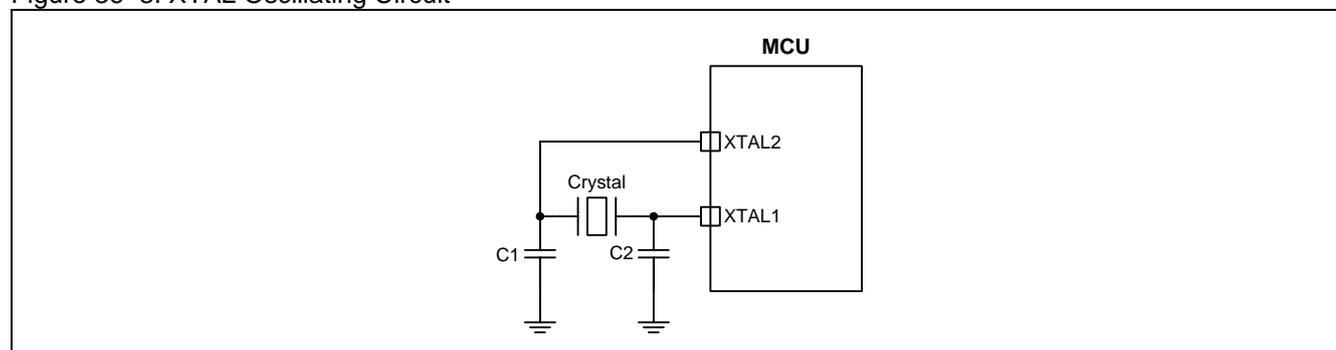
Table 36–1. Reference Capacitance of C1 & C2 for crystal oscillating circuit
