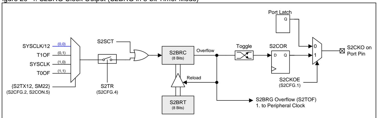
Figure 20–5. S2BRG Clock Output (S2BRG for UART Mode)
