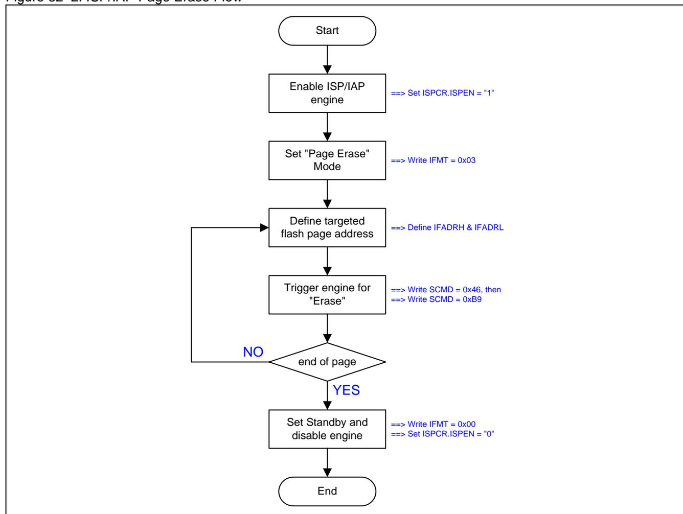
[Figure 32–3](#) shows the demo code of the ISP/IAP page erase operation.
