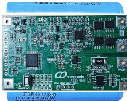
Figure 2-3 EVM actual connection of the cells figure
