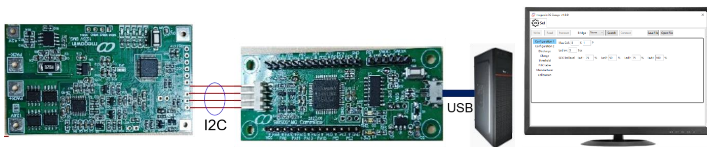
Figure 3-1 Hardware connection overview figure
