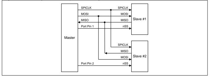
Figure 18-4. SPI single master multiple slaves configuration
