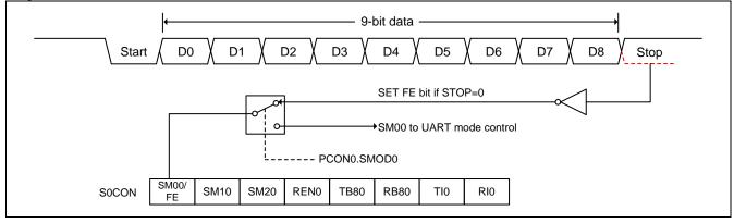
Figure 17-7. UART0 Frame Error Detection
