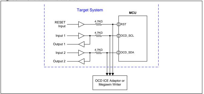
Figure 32-4. ICP and OCD Interface Circuit
