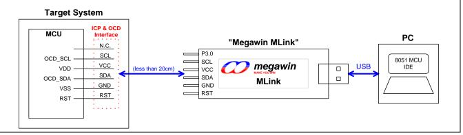
Figure 32-8. System Diagram for the ICE Function
