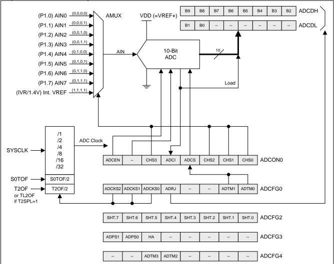
Figure 25-1. ADC Block Diagram
