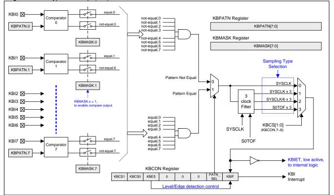
Figure 22-1. Keypad Interrupt (KBI) structure
