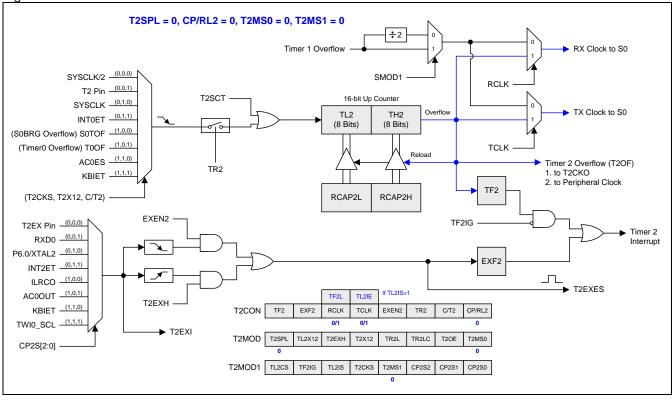
Figure 15-21. Timer 2 in Baud-Rate Generator Mode
