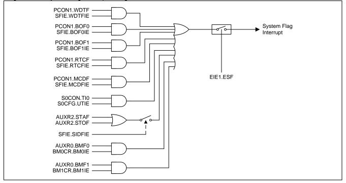
Figure 14-2. System flag interrupt configuration
