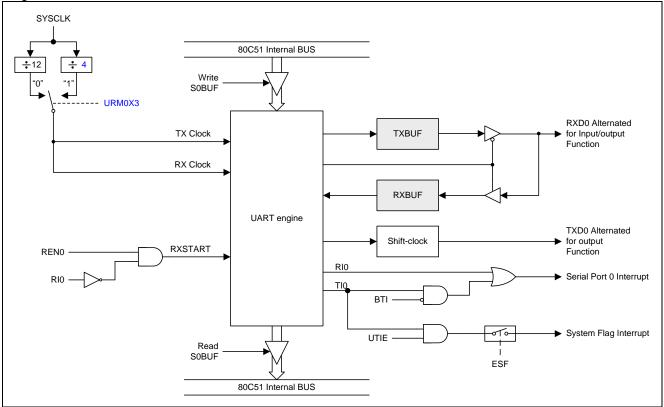
Figure 17-3. Serial Port 0 Mode 0
