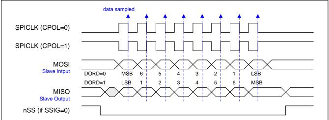
Figure 18-8. SPI Master Transfer Format with CPHA=0
