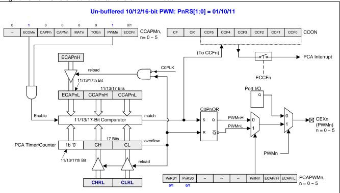
Figure 16-10. PCA0 Un-buffered10/12/16-bit PWM Mode
