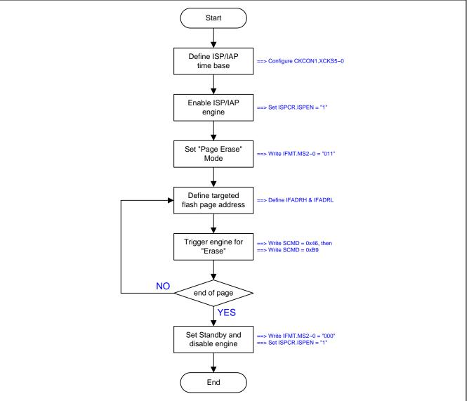
Figure 28-3 shows the demo code of the ISP/IAP page erase operation.
