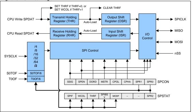
Figure 18-1. SPI Block Diagram
