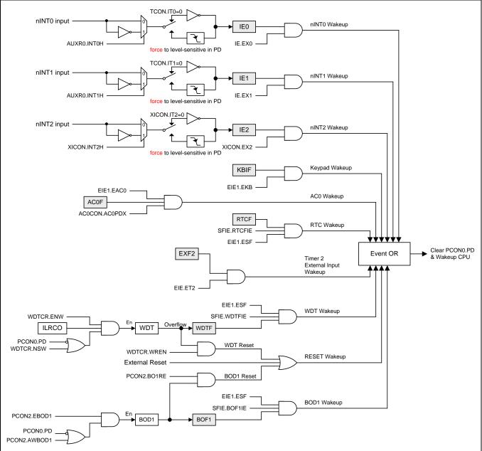
Figure 12-2. Wakeup structure of Power Down mode
