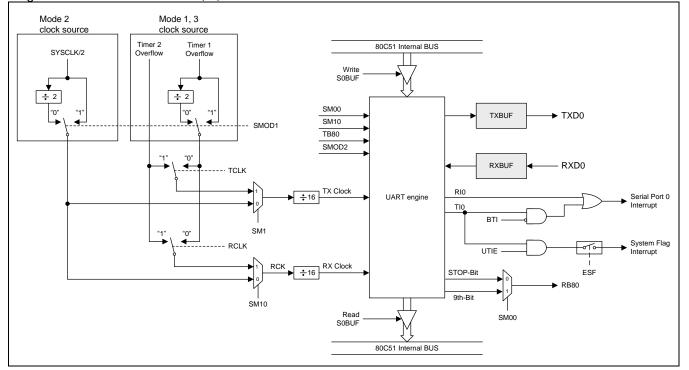
Figure 17-6. Serial Port Mode 1, 2, 3
