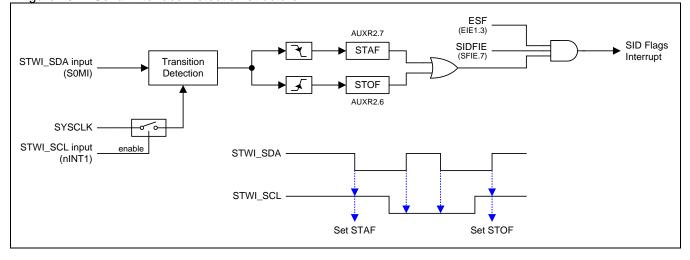
Figure 20-1. Serial Interface Detection structure
