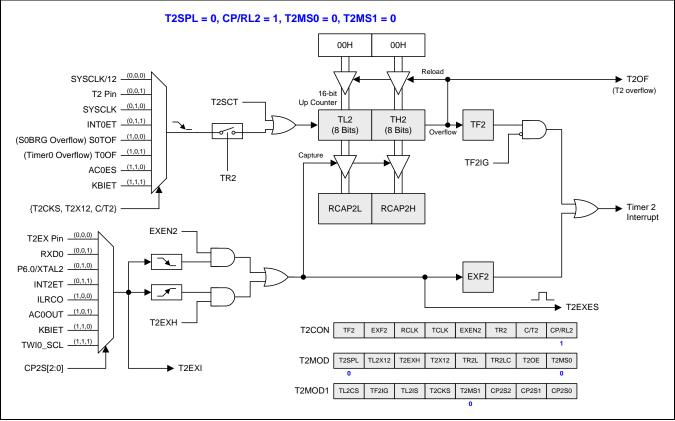
Figure 15-14. Timer 2 Mode 2 Structure (Capture Mode)
