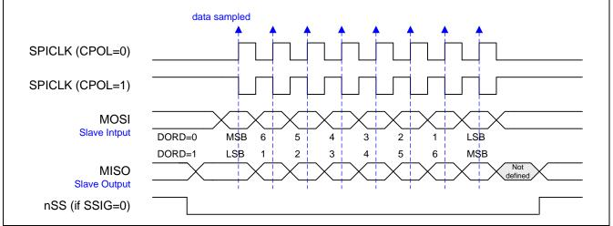
Figure 18-7. Slave Transfer Format with CPHA=1
