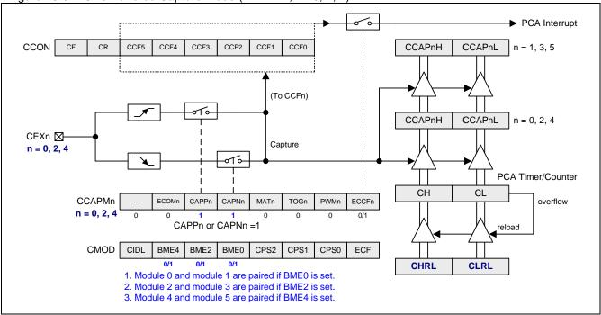
Figure 16-5. PCA0 Buffered Capture Mode (BMEn=1, n= 0, 2, 4)
