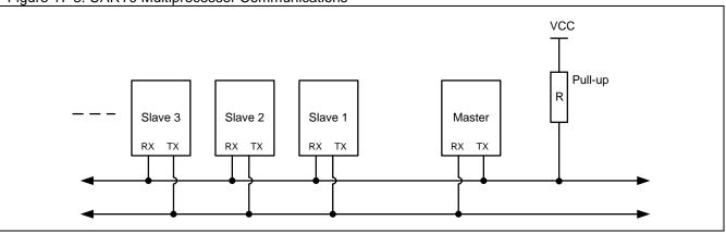
Figure 17-8. UART0 Multiprocessor Communications
