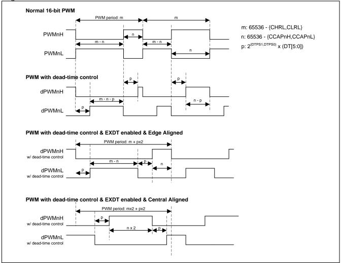
Figure 16–15. PWM Waveform with Dead-Time Control
