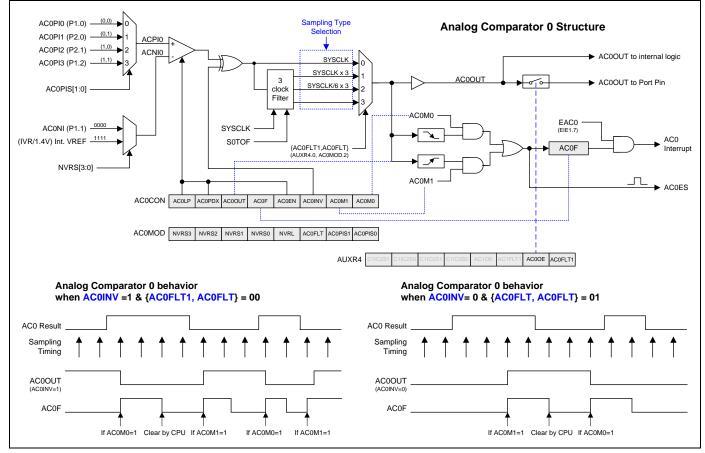
Figure 26-1. Analog Comparator 0 Block Diagram
