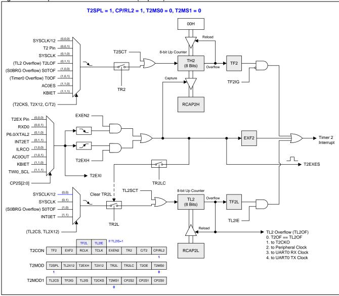
Figure 15-18. Split Timer 2 Mode 2 Structure (Capture)
